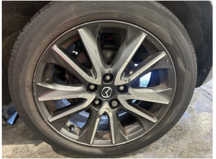
10: Wheel nsr Scratched Over 50mm
