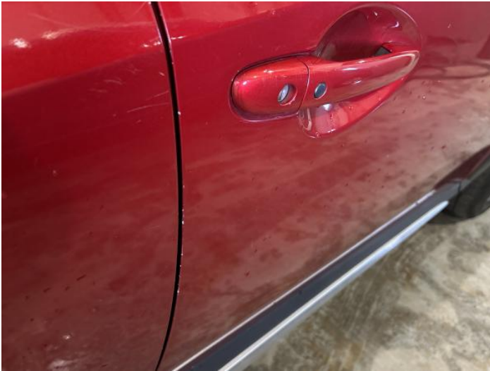
3: Door osf Chipped Edge Chip
