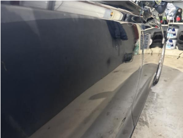
15: Door osr Dented Between 10mm + 30mm
