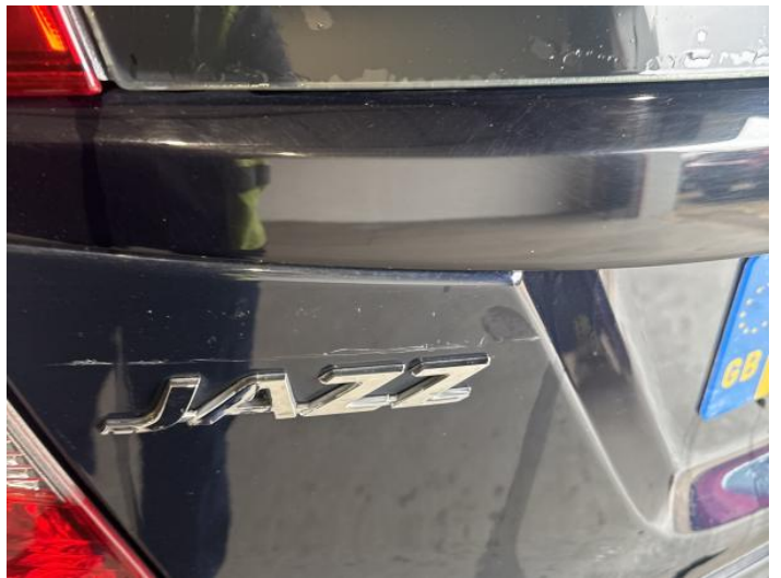
12: Boot Lid Scratched Over 25mm Thru Paint
