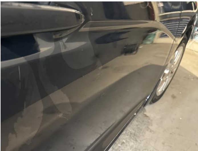
17: Door osf Dented Over 2 UpTo 10mm
