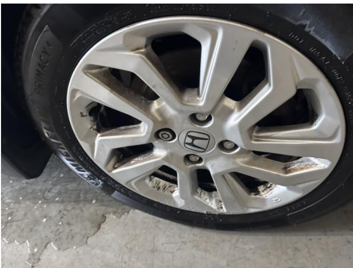
19: Wheel osf Scratched Over 50mm
