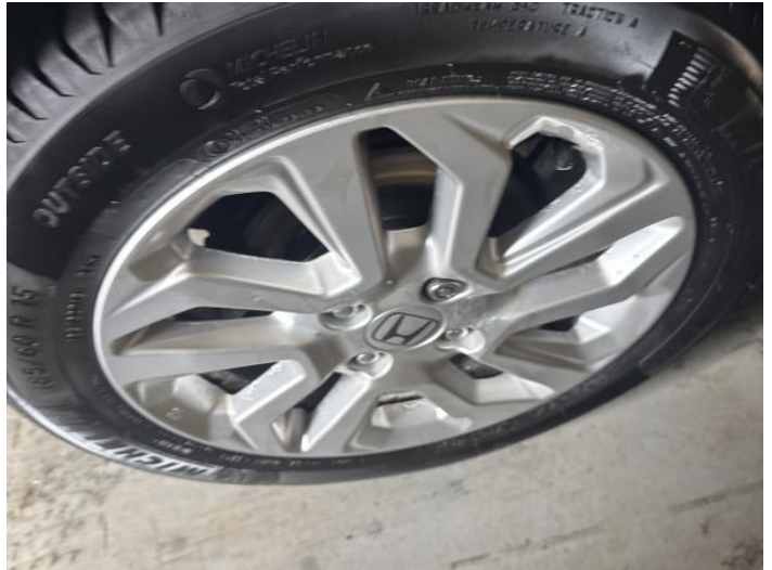
16: Wheel osr Scratched Over 50mm
