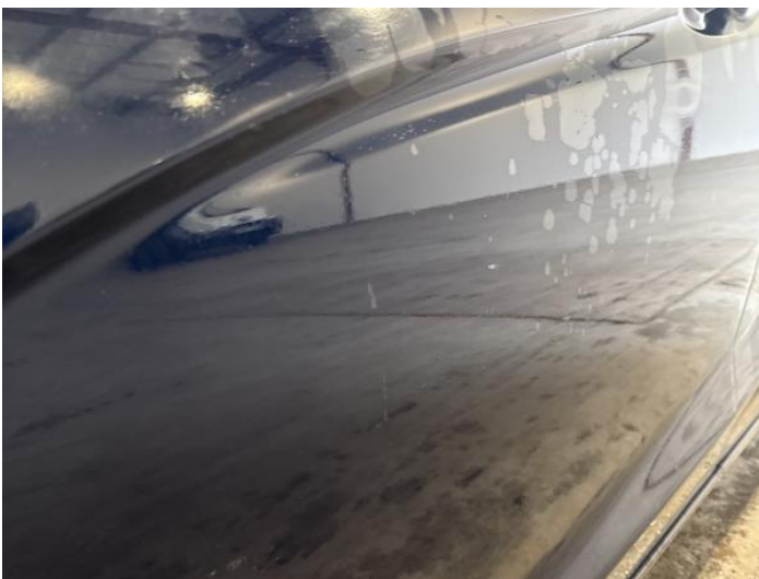
7: Door nsf Dented Over 2 UpTo 10mm
