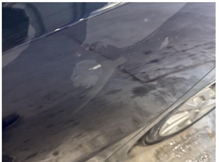
8: Door nsr Scratched Over 25mm Thru Paint
