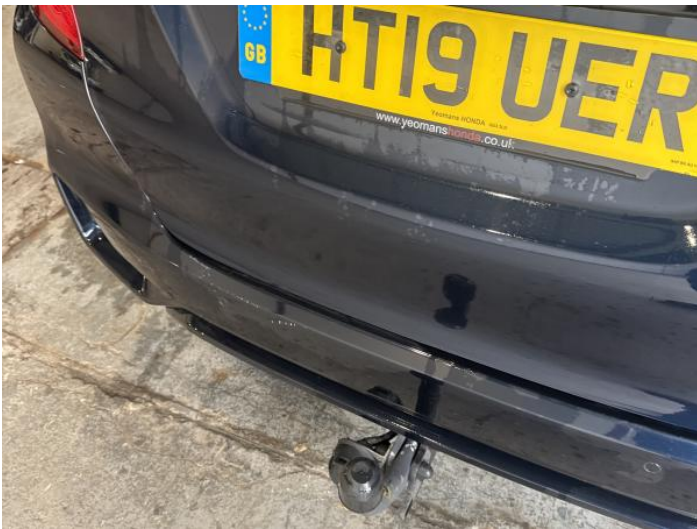
11: Bumper Rear Scratched Over 100mm Thru Paint
