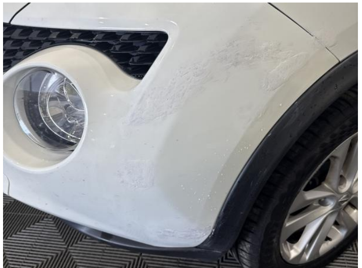
2: Bumper Front Scratched Over 100mm Thru Paint
