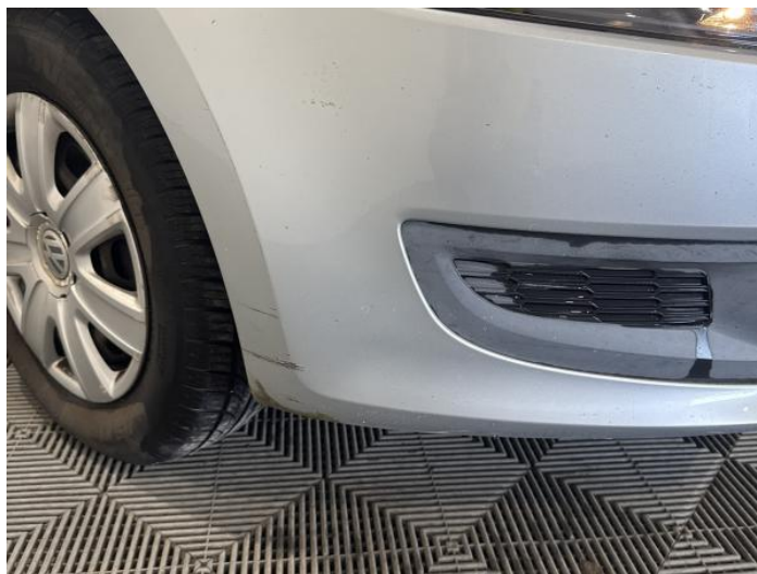
2: Bumper Front Scratched Over 100mm Thru Paint
