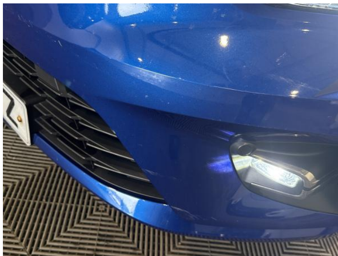
2: Bumper Front Scratched Over 100mm Thru Paint
