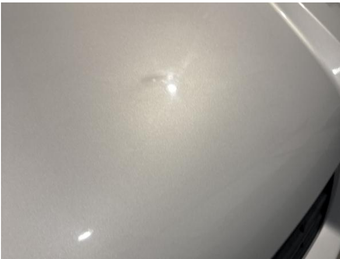
11: Bonnet Poor Previous Repair Poor Paint
