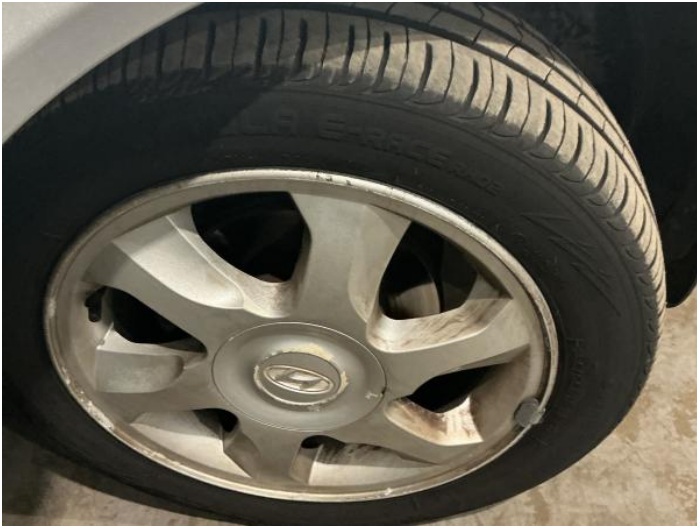
15: Wheel nsf Scratched Over 50mm
