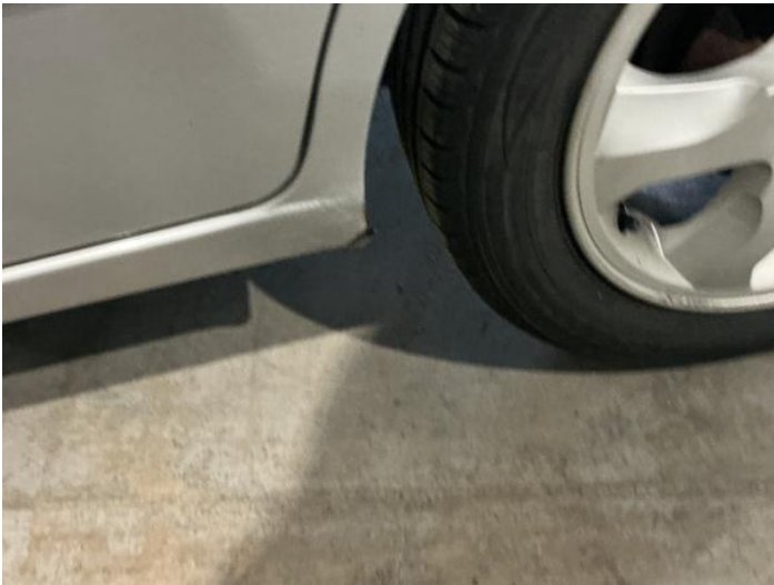
17: Sill ns Rusted Over 5mm
