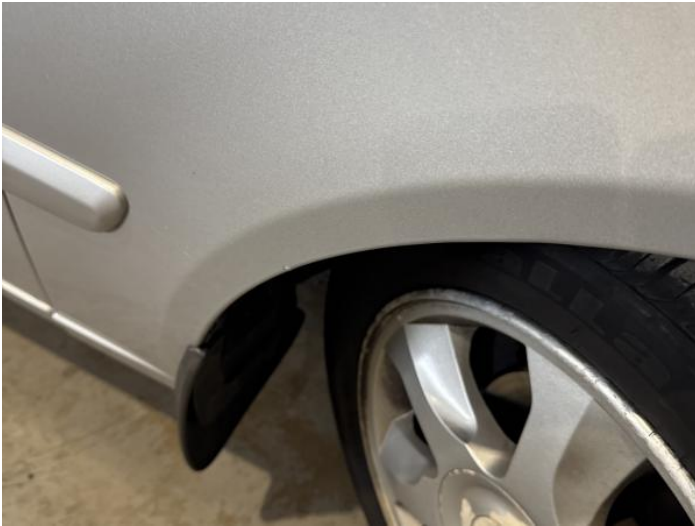
9: Wing osf Chipped 1 To 5
