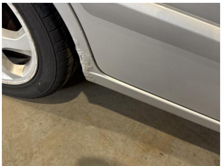
8: Sill os Rusted Over 5mm
