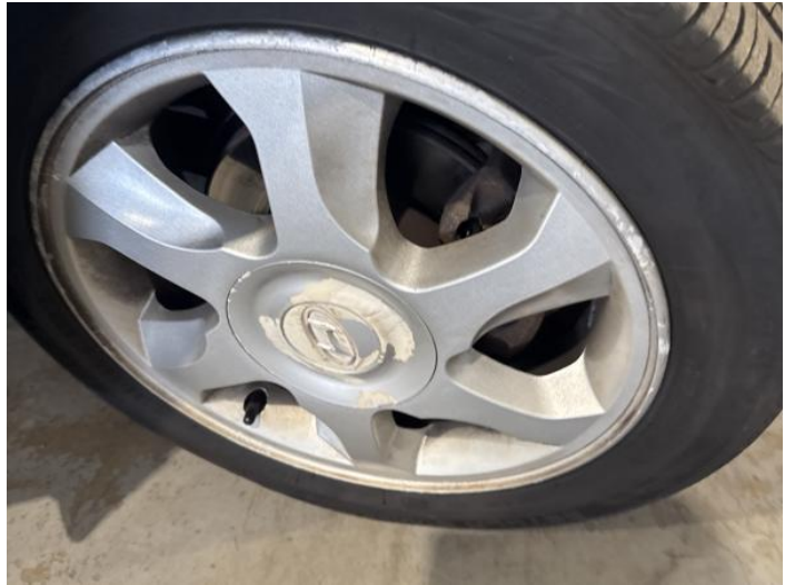
10: Wheel osf Scratched Over 50mm
