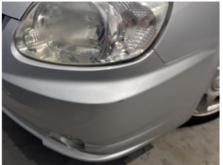
12: Bumper Front Scratched 25 to 100mm Thru Paint
