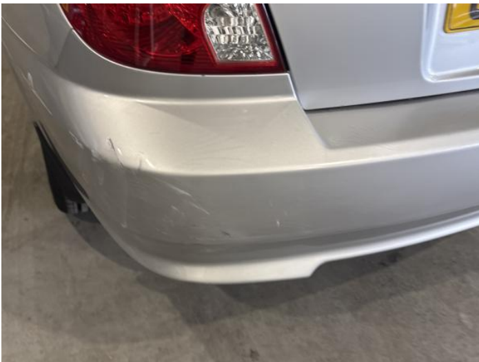
1: Bumper Rear Poor Previous Repair Rippled Up To 30%
