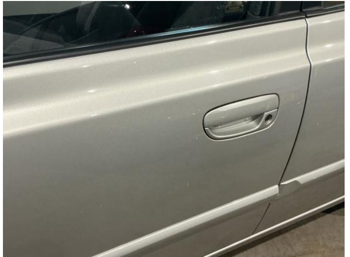
16: Door nsf Dented Between 10mm + 30mm
