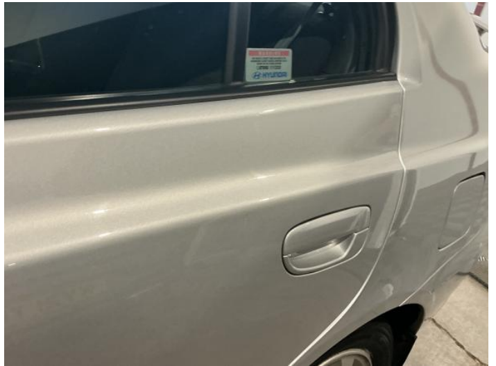
18: Door nsr Dented Between 10mm + 30mm
