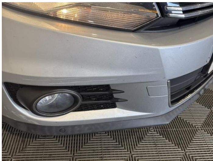
2: Bumper Front Scratched Over 100mm Thru Paint
