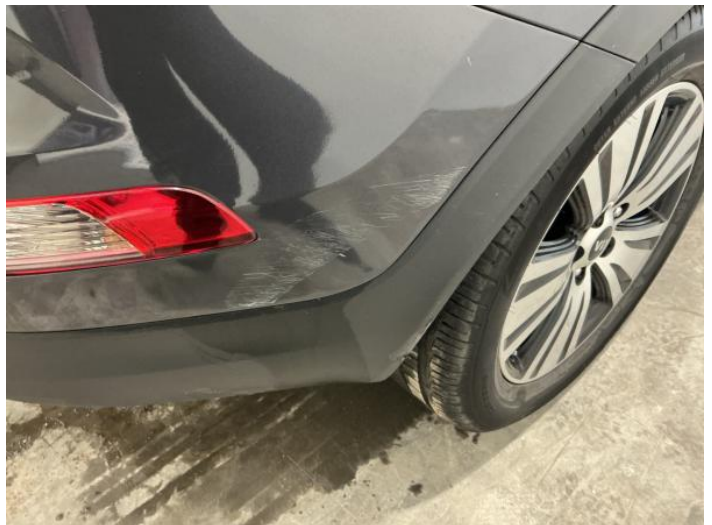
8: Bumper Rear Scratched 25 to 100mm Thru Paint
