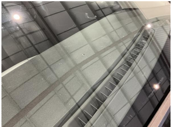
16: Screen Front Chipped UpTo 10mm
