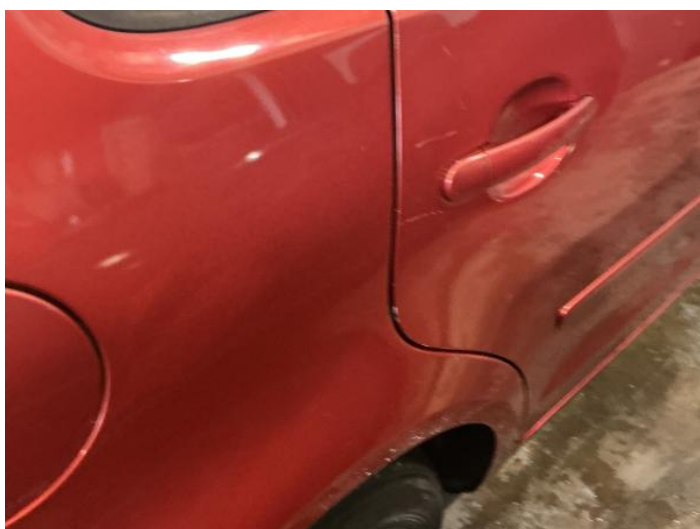
17: Qtr Panel osr Dented With Paint Damage
