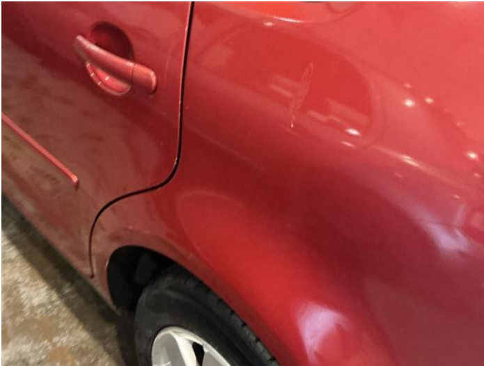
3: Qtr Panel nsr Dented With Paint Damage
