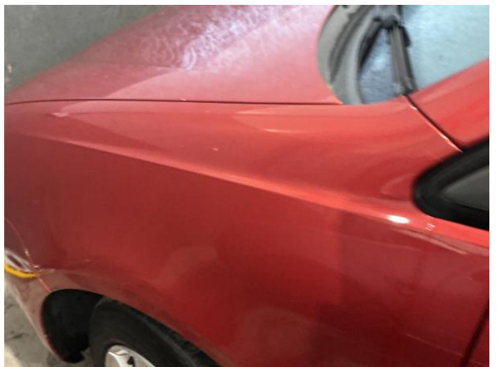
8: Wing nsf Dented With Paint Damage
