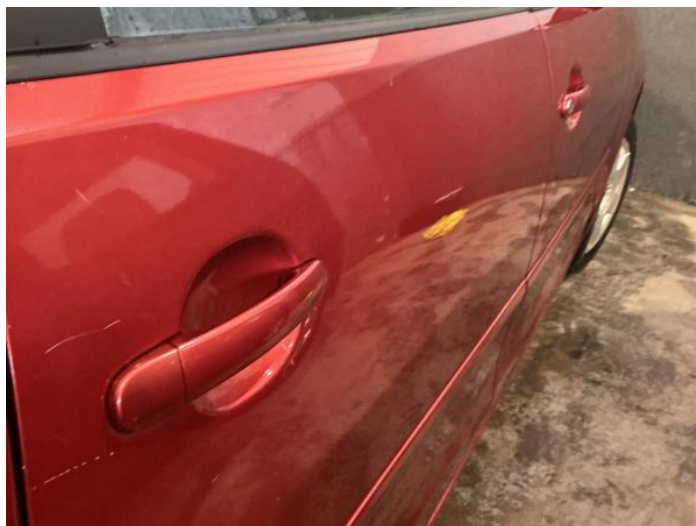
16: Door osr Scratched Over 25mm Thru Paint
