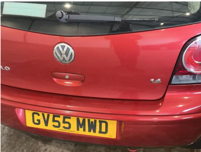
1: Bumper Rear Scratched Over 100mm Thru Paint
