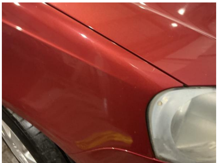
12: Wing osf Dented Over 2 UpTo 10mm
