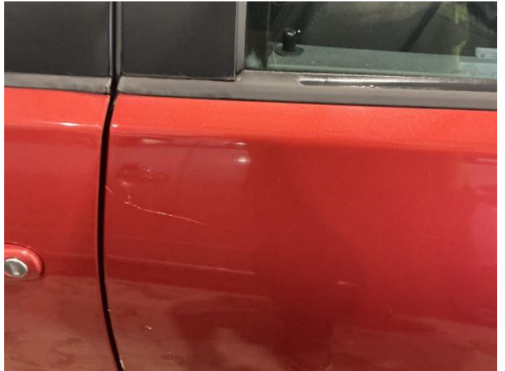
4: Door nsr Scratched Over 25mm Thru Paint
