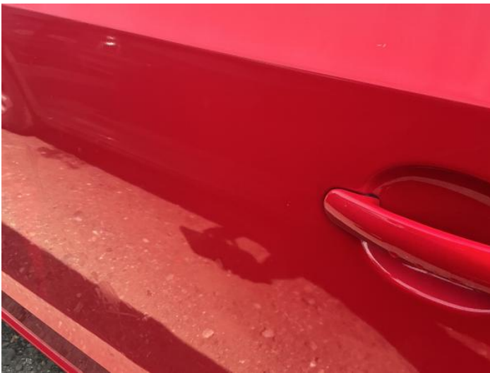
5: Door nsf Poor Previous Repair Poor Paint
