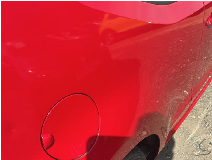
9: Qtr Panel osr Dented 2 Or Less UpTo 10mm
