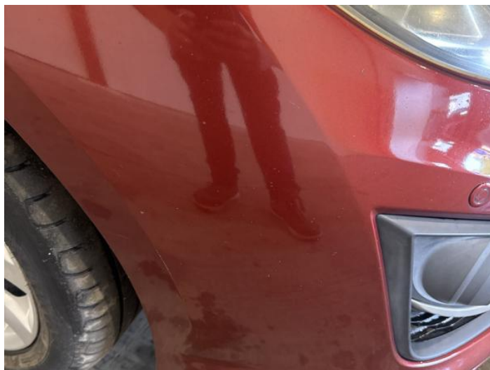
2: Bumper Front Scratched Over 100mm Thru Paint
