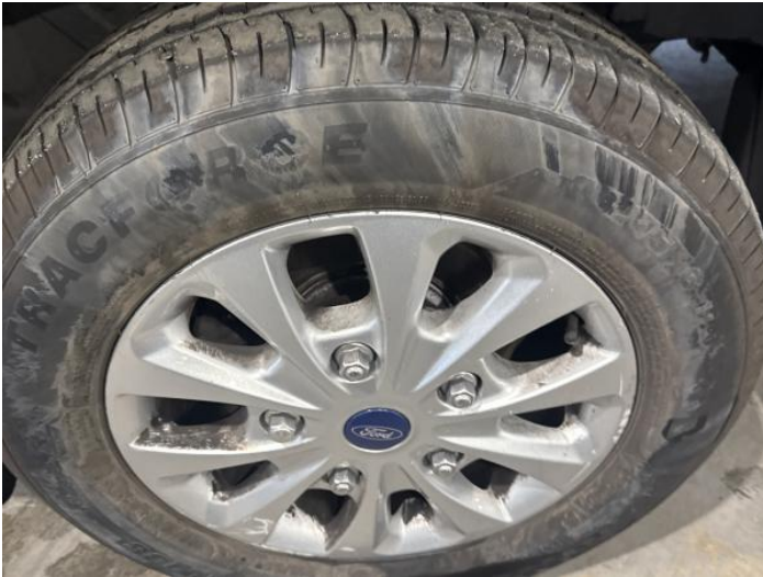
15: Wheel osr Scratched Over 50mm
