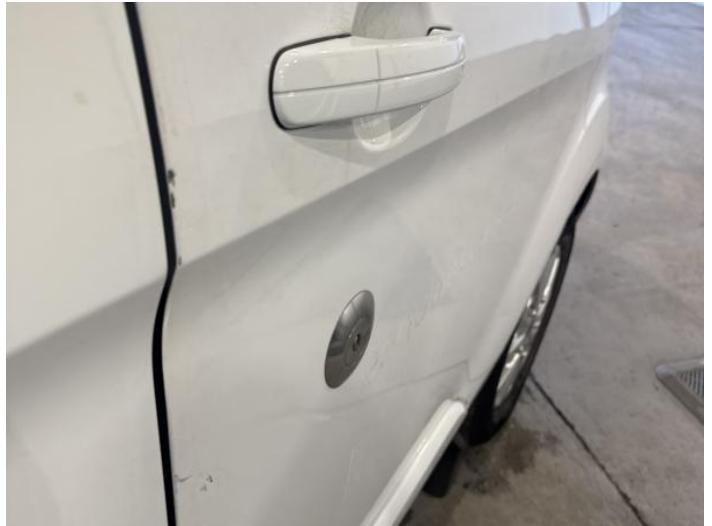
16: Door osf Scratched Over 25mm Thru Paint
