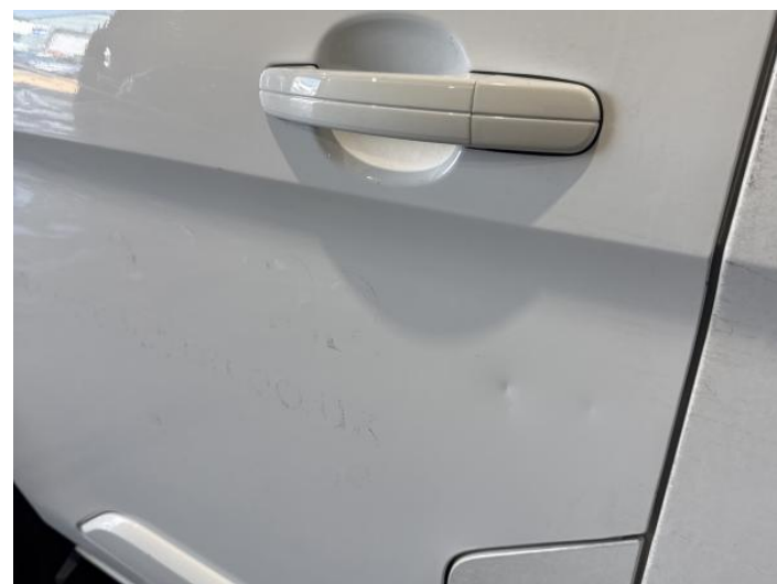
7: Door nsf Dented With Paint Damage
