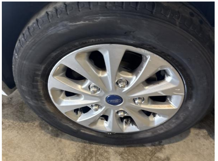
6: Wheel nsf Scratched Over 50mm
