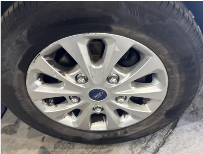
17: Wheel osf Scratched Over 50mm
