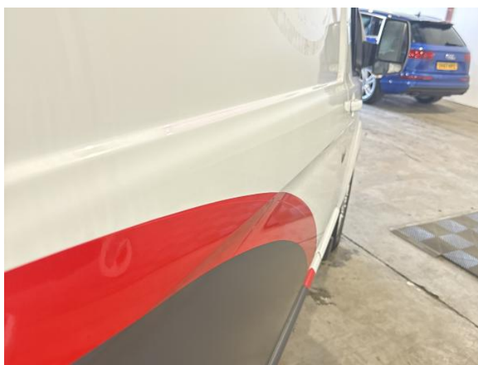
14: Qtr Panel osr Dented Over 30mm
