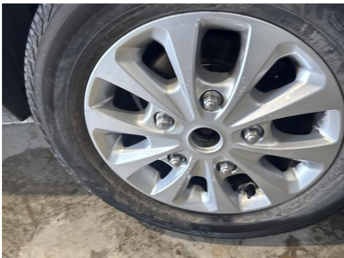
9: Wheel nsr Scratched Over 50mm
