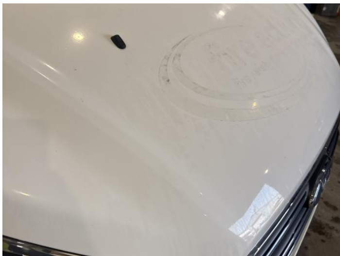
1: Bonnet Poor Previous Repair Poor Paint
