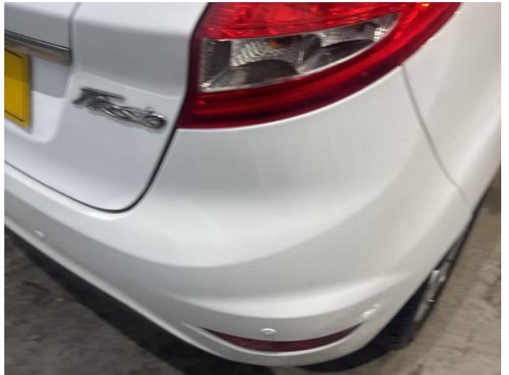
12: Bumper Rear Poor Previous Repair Poor Colour
