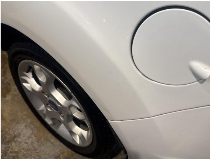
11: Qtr Panel nsr Dented With Paint Damage
