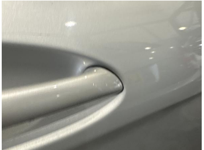
10: Door osf Scratched Over 25mm Thru Paint
