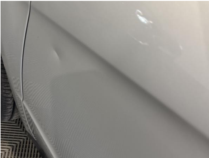
5: Door nsf Dented With Paint Damage
