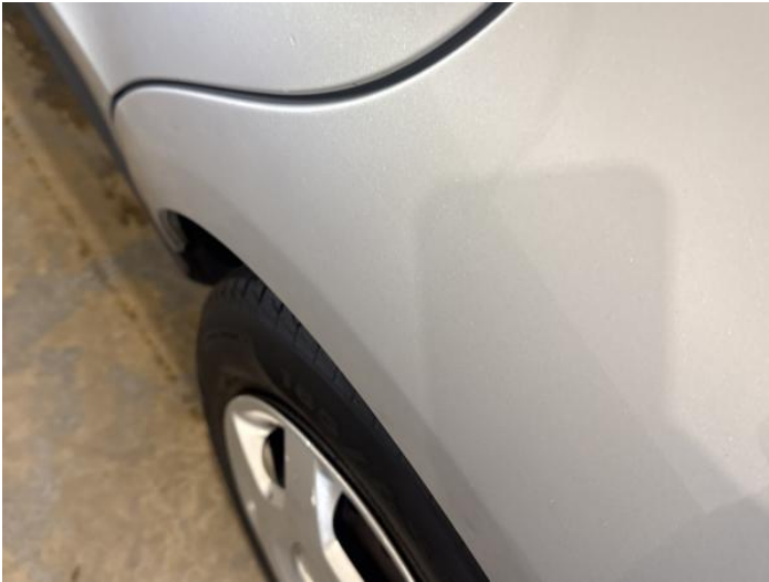
3: Qtr Panel nsr Dented Over 2 UpTo 10mm
