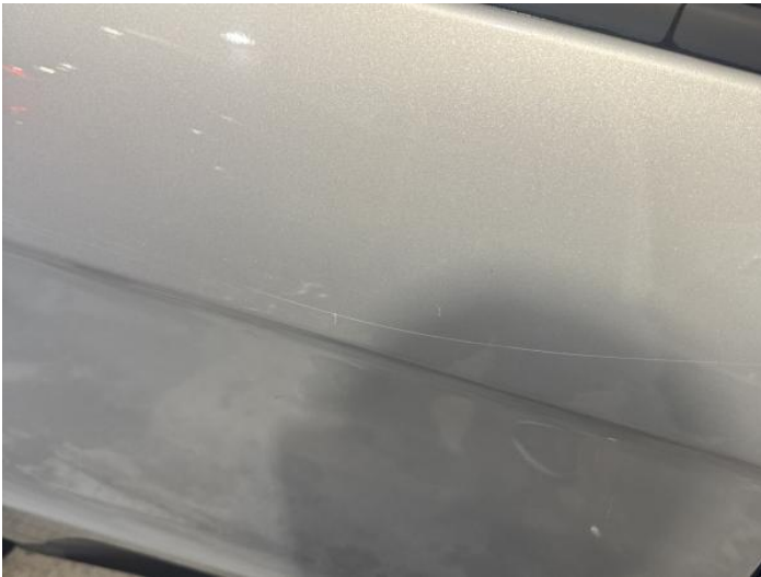
11: Door osr Scratched Over 25mm Thru Paint
