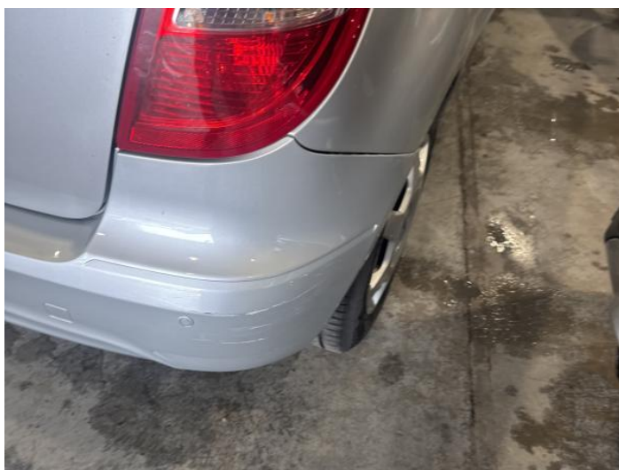
1: Bumper Rear Scratched Over 100mm Thru Paint
