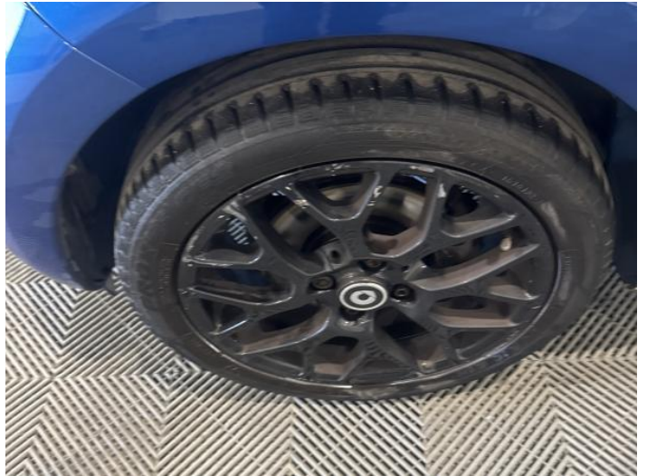
4: Wheel nsf Scratched Over 50mm
