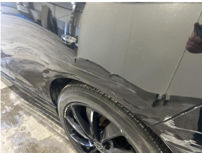
7: Qtr Panel nsr Dented With Paint Damage
