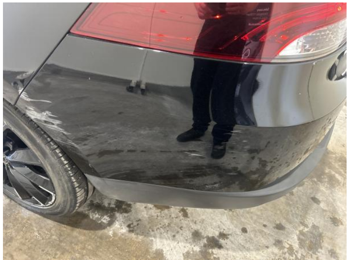
6: Bumper Rear Scratched 25 to 100mm Thru Paint
