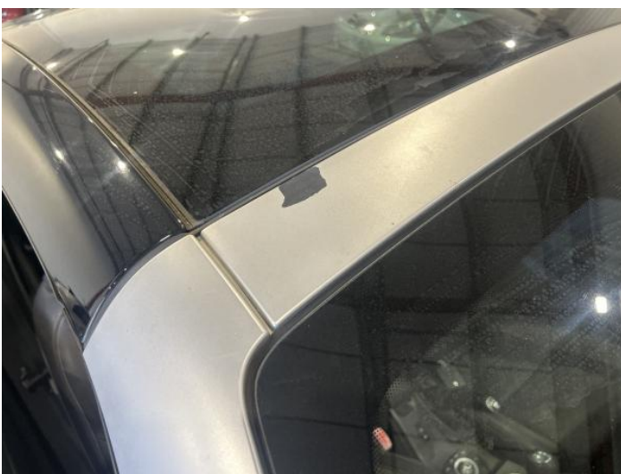
13: Roof Poor Previous Repair Paint Flake
