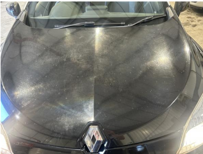
11: Bonnet Poor Previous Repair Poor Paint
