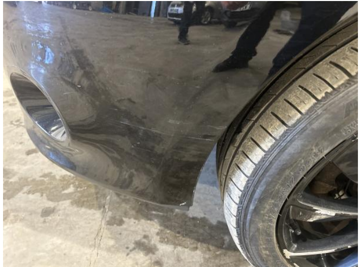
10: Bumper Front Scratched 25 to 100mm Thru Paint
