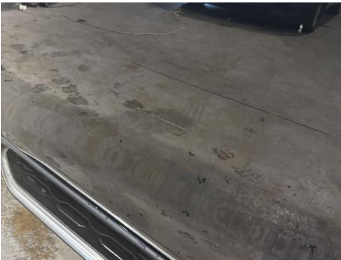
5: Door nsf Scratched Over 25mm Thru Paint
