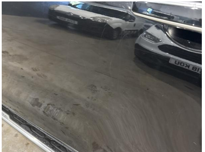
6: Door nsr Scratched Over 25mm Thru Paint
