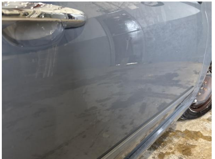
6: Door osf Dented Over 2 UpTo 10mm
