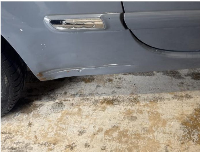
5: Sill os Dented With Paint Damage
