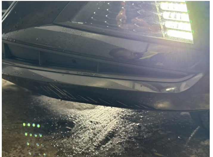
2: Bumper Front Scratched Over 100mm Thru Paint
