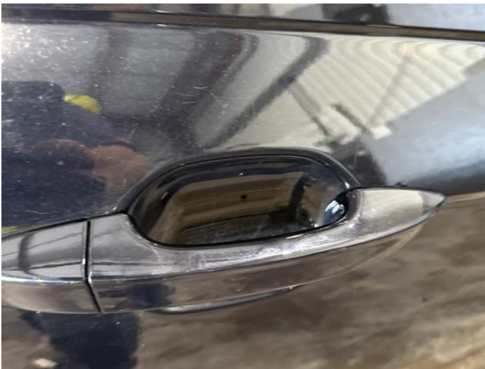
11: Door osf Scratched UpTo 25mm Thru Paint
