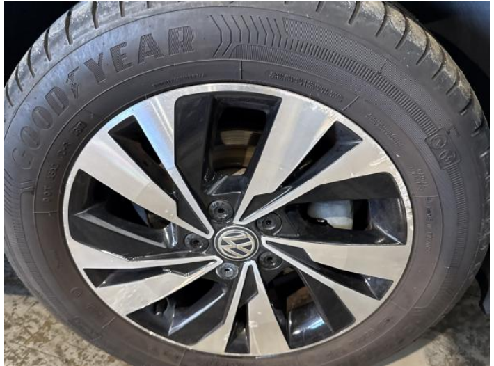
10: Wheel osf Scratched Over 50mm
