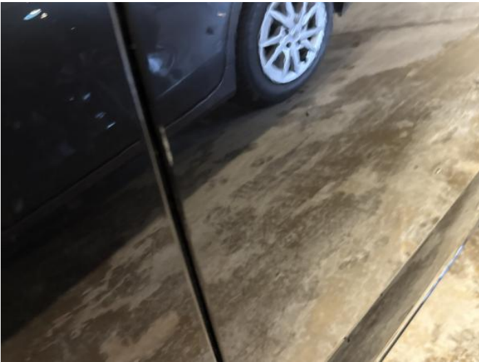
5: Door nsr Chipped Edge Chip
