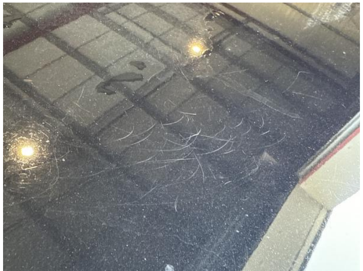
12: Roof Scratched Over 25mm Thru Paint
