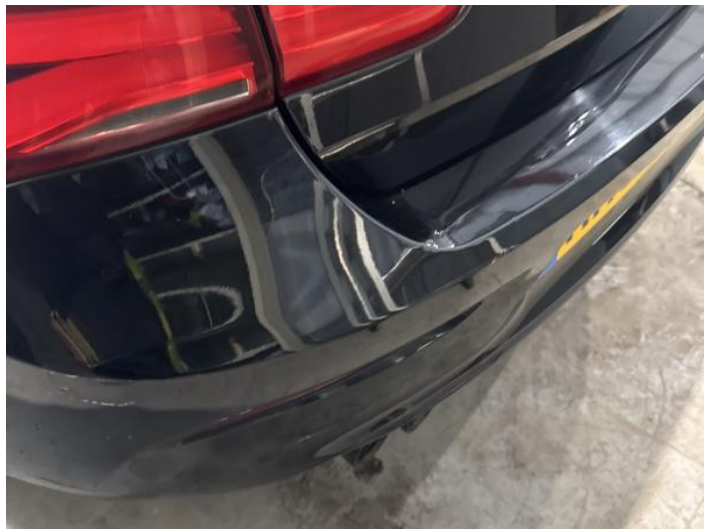
12: Bumper Rear Poor Previous Repair Rippled UpTo 30%
