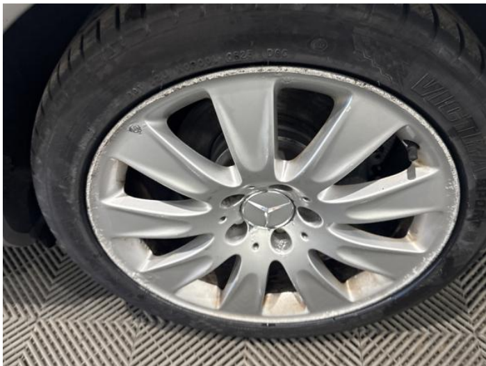
9: Wheel nsr Scratched Over 50mm
