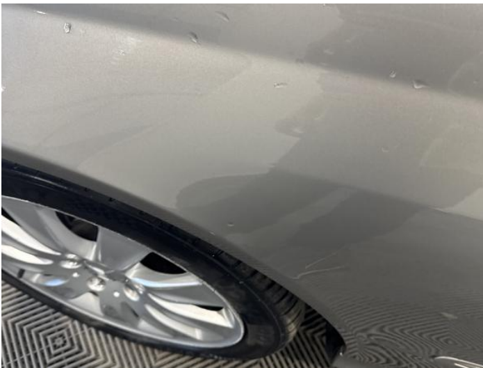
5: Wing nsf Dented Over 2 UpTo 10mm
