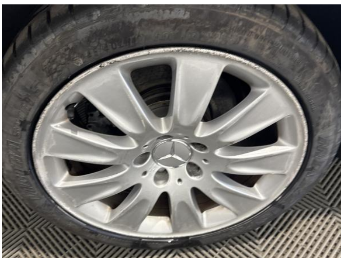
13: Wheel osr Scratched Over 50mm
