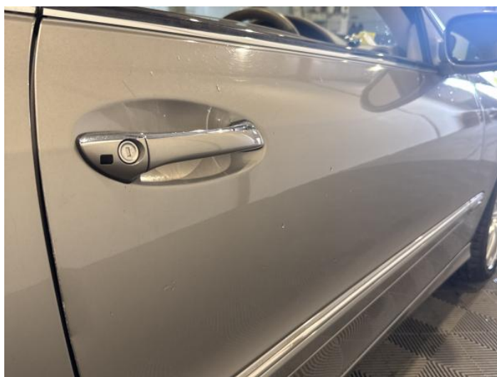
14: Door osf Dented Over 30mm
