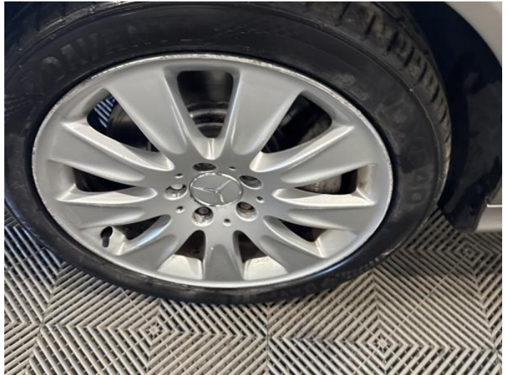
4: Wheel nsf Scratched Over 50mm
