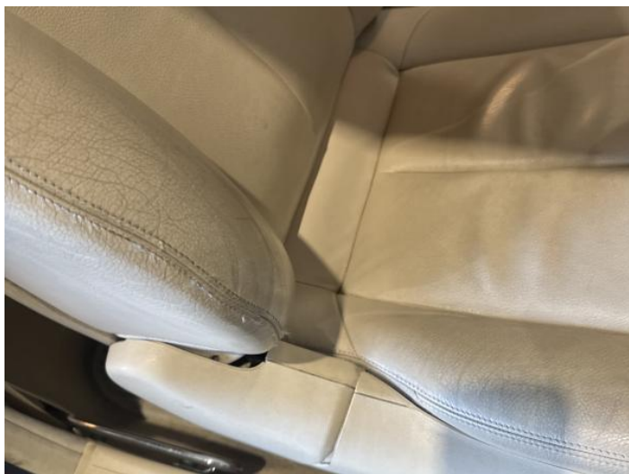
1: Seat Base Cover osf Torn UpTo 3mm
