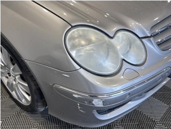
3: Bumper Front Scratched Over 100mm Thru Paint
