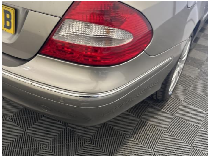
10: Bumper Rear Scratched Over 100mm Thru Paint
