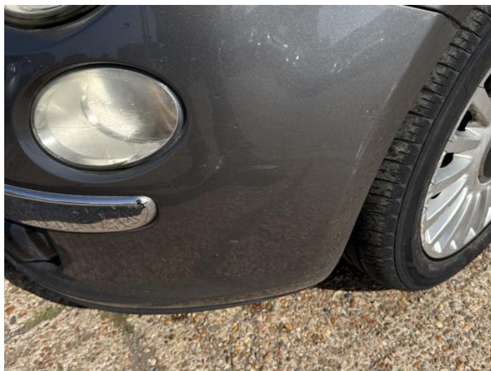
2: Bumper Front Scratched Over 100mm Thru Paint
