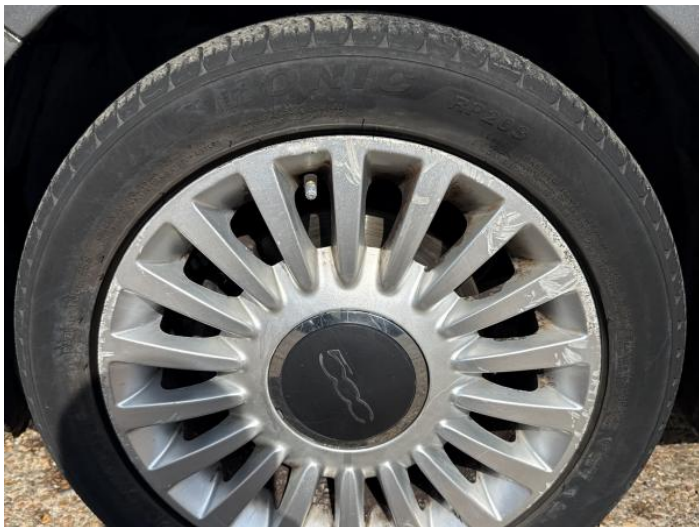
3: Wheel nsf Scratched Over 50mm
