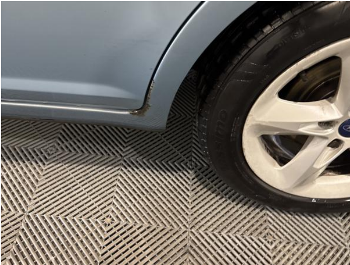
9: Qtr Panel nsr Rusted Over 5mm
