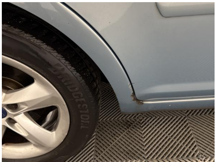
14: Qtr Panel osr Rusted Over 5mm
