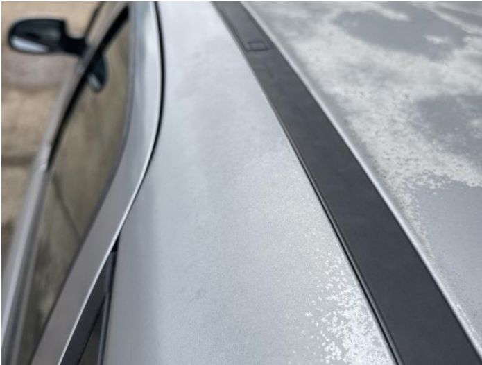
15: D Post ns Poor Previous Repair Poor Paint
