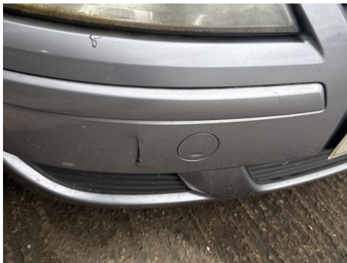
2: Bumper Front Cracked Over 25mm
