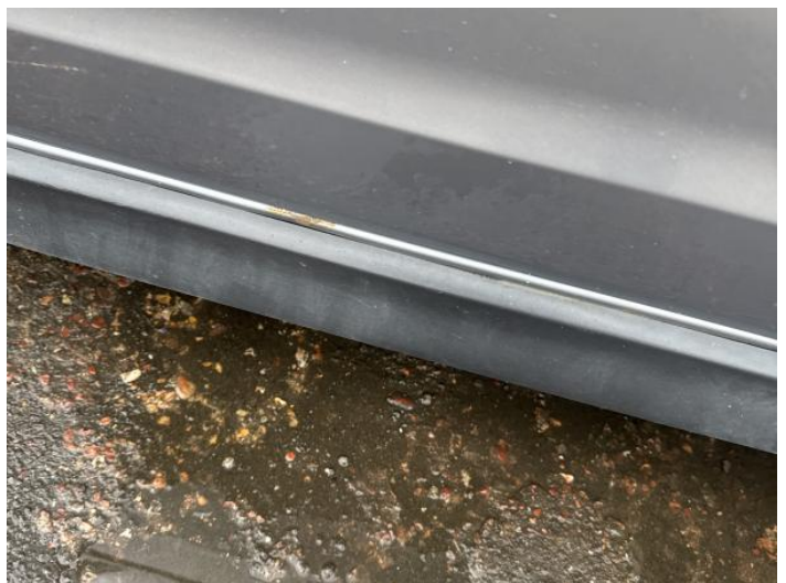
8: Sill ns Rusted Over 5mm
