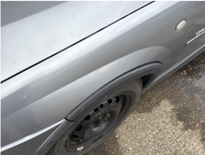
5: Wing nsf Poor Previous Repair Poor Paint
