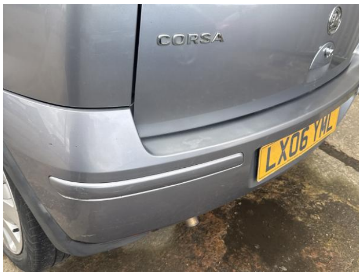
12: Bumper Rear Poor Previous Repair Paint Flake
