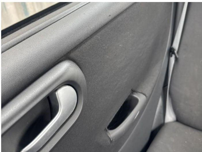
27: Door Pad osr Torn Over 10mm
