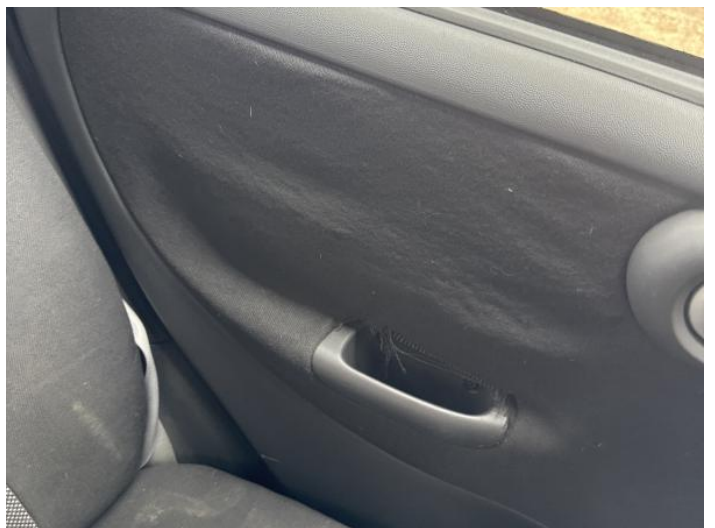
26: Door Pad nsr Torn Over 10mm
