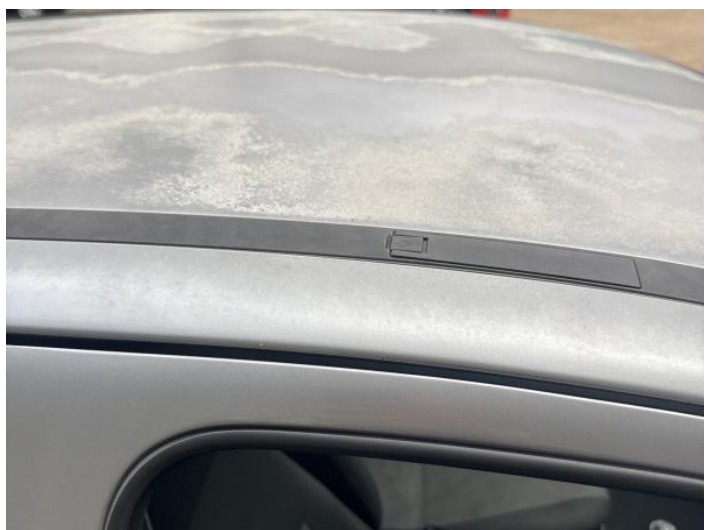
20: A Post os Poor Previous Repair Poor Paint
