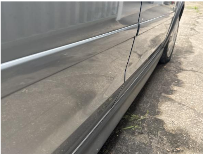
17: Door osr Dented Over 30mm
