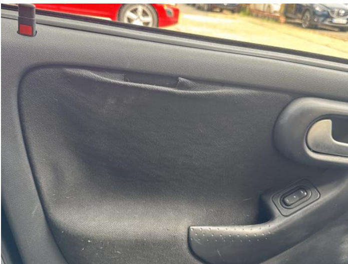
25: Door Pad nsf Torn Over 10mm
