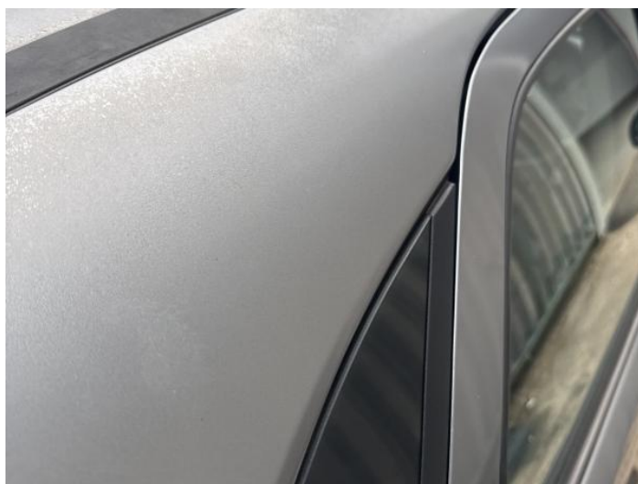
14: D Post os Poor Previous Repair Poor Paint
