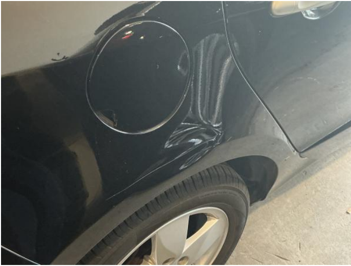
3: Qtr Panel osr Dented With Paint Damage
