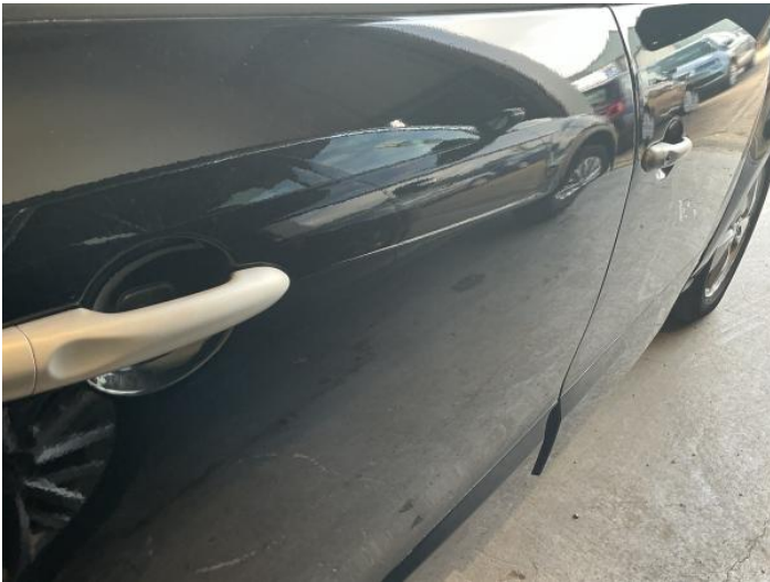
5: Door osr Dented Over 30mm
