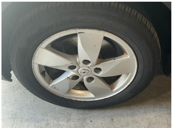
14: Wheel nsf Scratched Over 50mm
