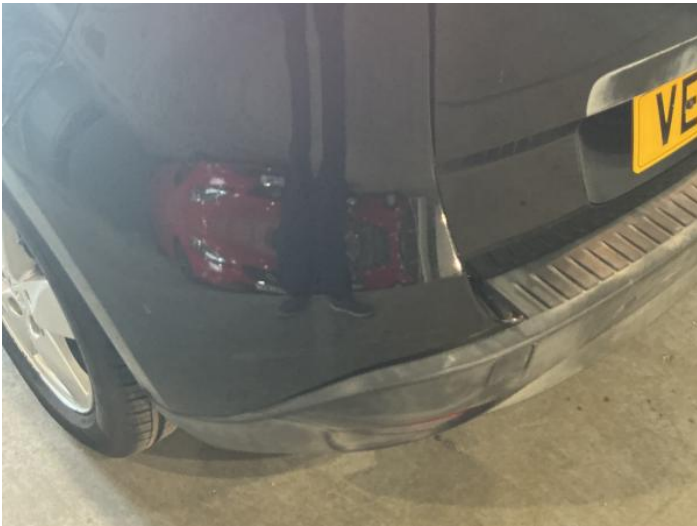
1: Bumper Rear Poor Previous Repair Poor Paint
