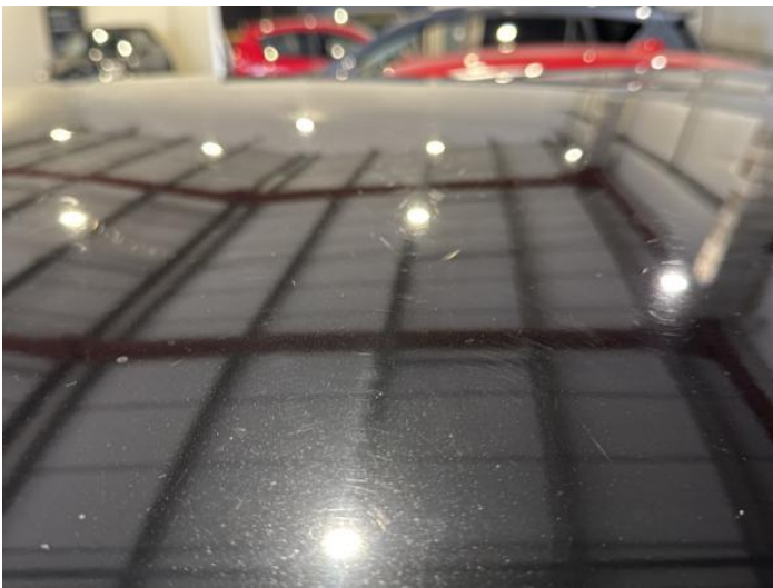
23: Roof Dented Over 30mm
