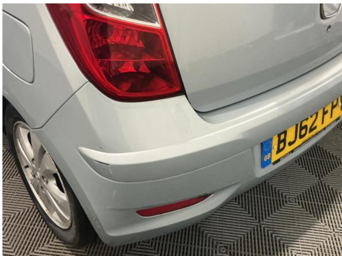
9: Bumper Rear Scratched Over 100mm Thru Paint
