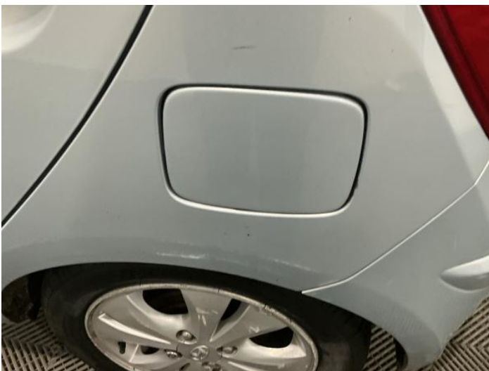
7: Qtr Panel nsr Dented With Paint Damage
