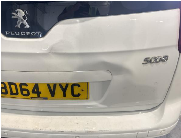
11: Boot Lid Dented Over 30mm
