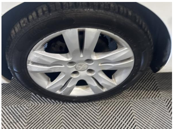
18: Wheel nsf Scratched Over 50mm
