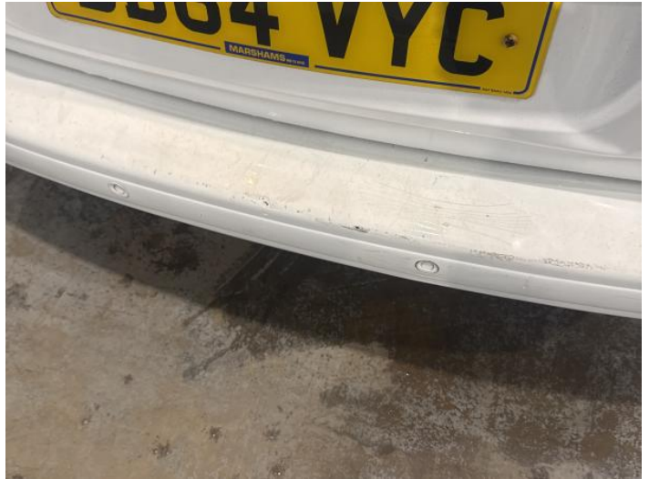
10: Bumper Rear Poor Previous Repair Rippled UpTo 30%
