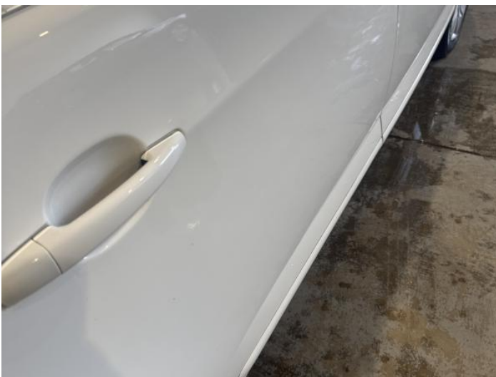
7: Door osr Dented 2 Or Less UpTo 10mm
