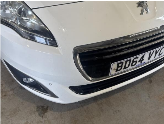
1: Bumper Front Scratched Over 100mm Thru Paint
