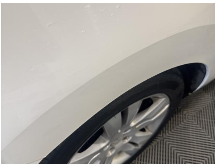
19: Wing nsf Scratched Over 25mm Not Thru Paint
