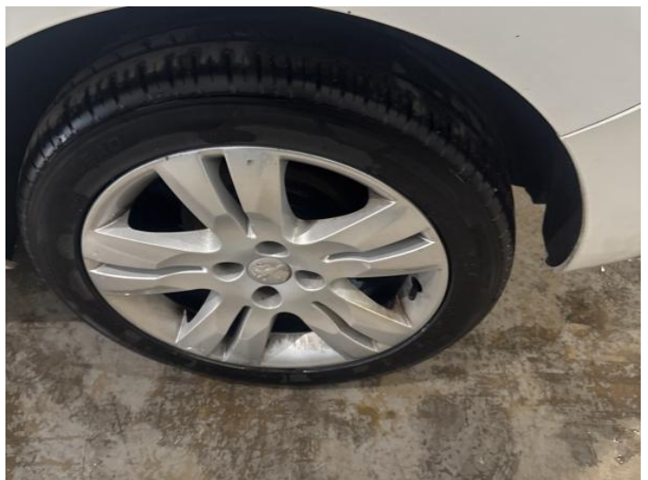
14: Wheel nsr Scratched Over 50mm
