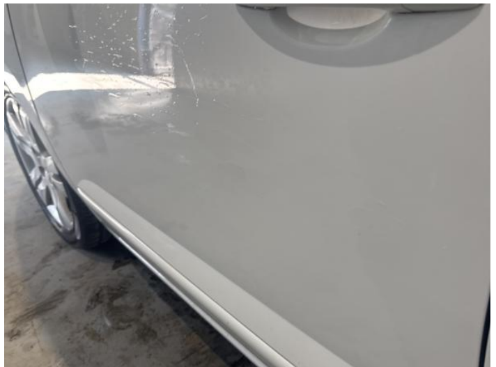
16: Door nsf Dented Over 2 UpTo 10mm
