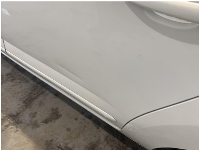
15: Door nsr Dented Over 30mm
