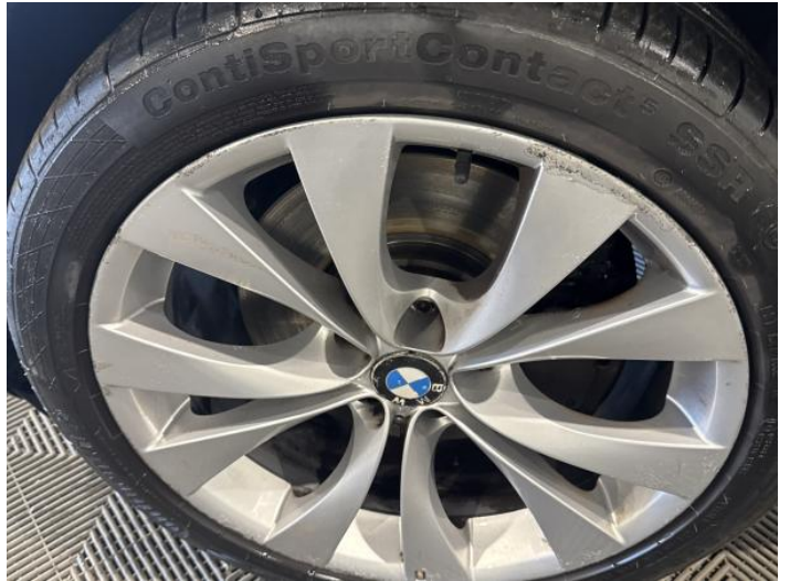
4: Wheel nsf Scratched Over 50mm
