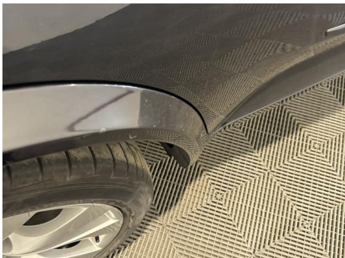
21: Qtr Panel Arch Extension os Scratched (Painted) Over 25mm Thru Paint
