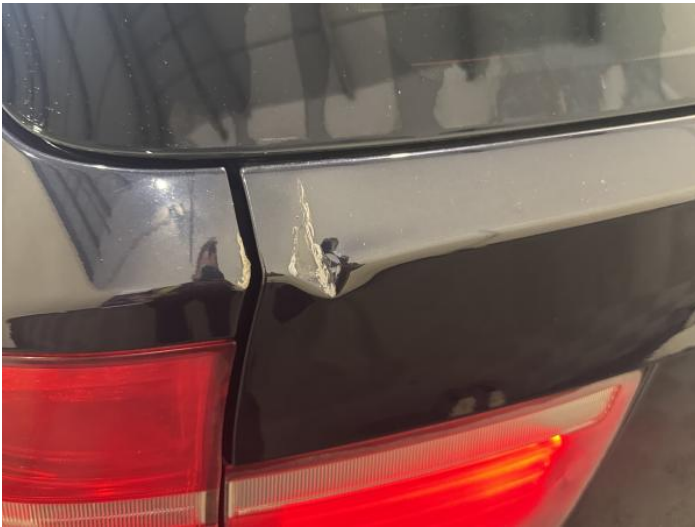
17: Boot Lid Dented With Paint Damage
