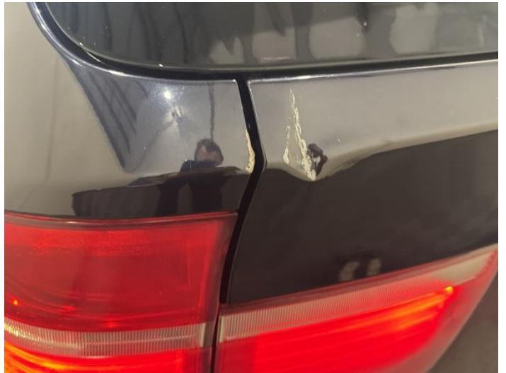
18: Qtr Panel nsr Dented With Paint Damage
