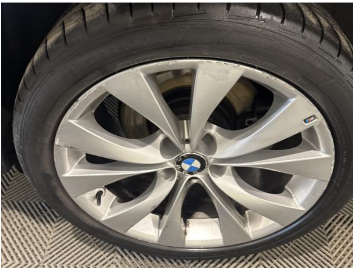
11: Wheel nsr Scratched Over 50mm
