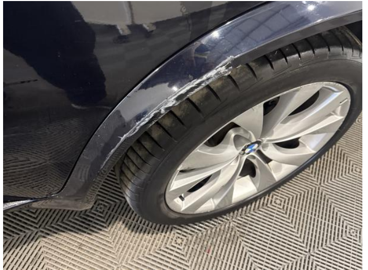
10: Qtr Panel Arch Extension ns Scratched (Painted) Over 25mm Thru Paint
