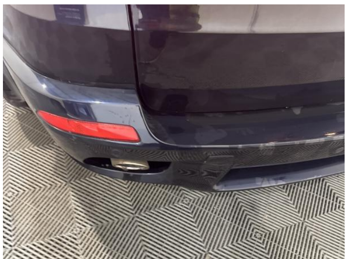
14: Bumper Rear Scratched Over 100mm Thru Paint
