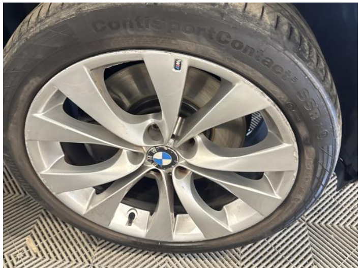
28: Wheel osf Scratched Over 50mm
