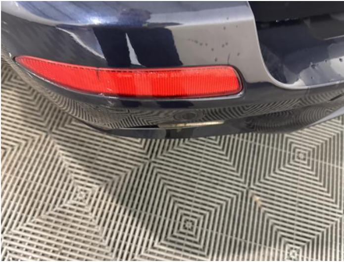
15: Bumper Reflector nsr Broken Replace
