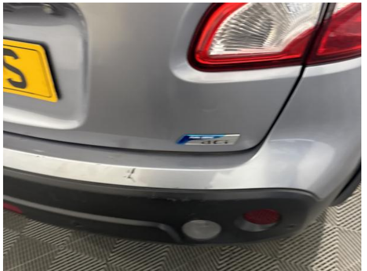
12: Bumper Rear Scratched Over 100mm Thru Paint
