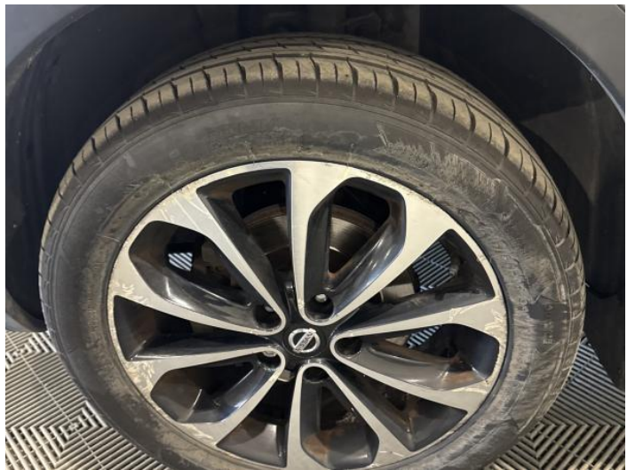
4: Wheel nsf Scratched Over 50mm
