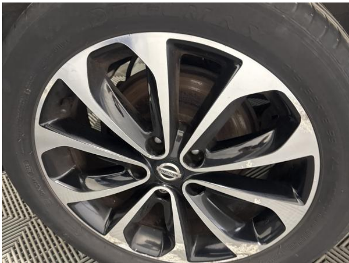
15: Wheel osr Scratched Over 50mm
