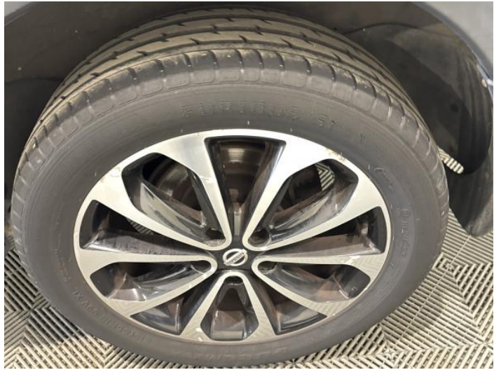
10: Wheel nsr Scratched Over 50mm
