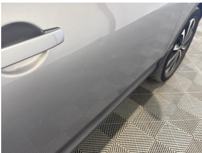
19: Door osf Dented With Paint Damage
