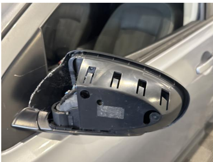
7: Door Mirror Assy nsf Broken Replace
