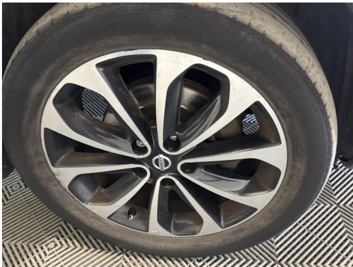
21: Wheel osf Scratched Over 50mm
