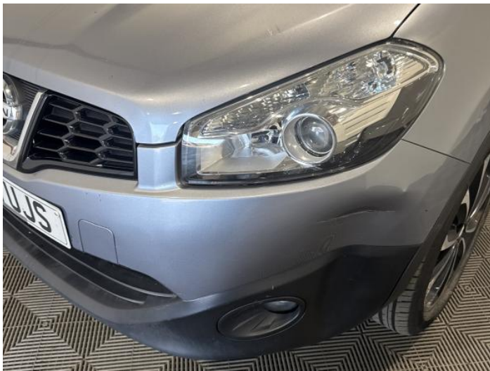
3: Bumper Front Dented With Paint Damage
