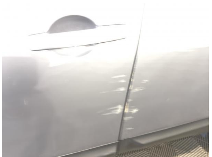
8: Door nsf Dented With Paint Damage
