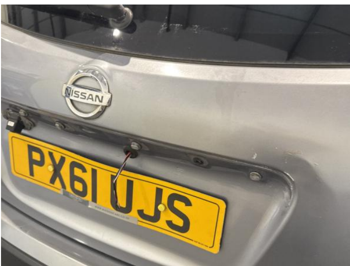
13: Boot Lid Dented With Paint Damage
