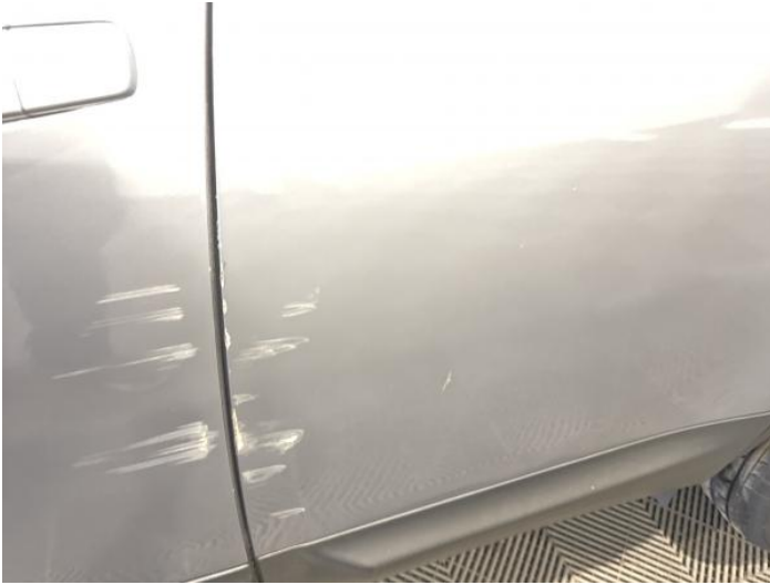
9: Door nsr Dented With Paint Damage
