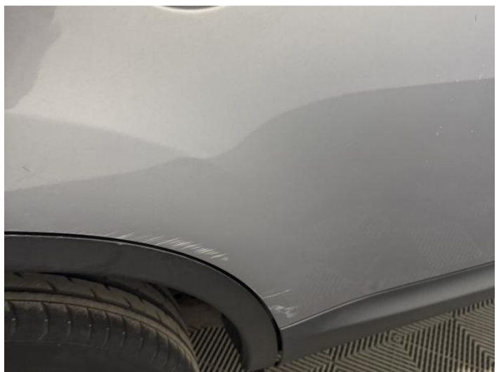
18: Door osr Dented With Paint Damage
