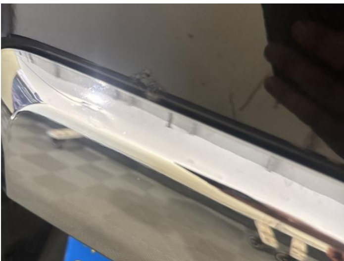
13: Boot Lid Rusted UpTo 5mm
