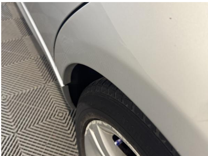
9: Qtr Panel nsr Dented Between 10mm + 30mm
