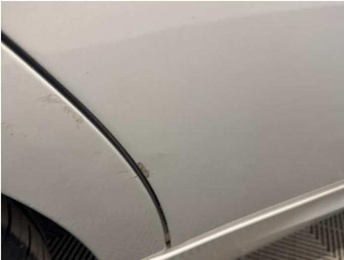
15: Door osr Scratched UpTo 25mm Thru Paint
