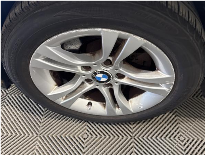
3: Wheel nsf Scratched Over 50mm
