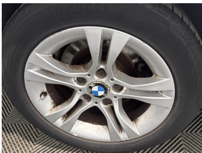
14: Wheel osr Scratched Over 50mm
