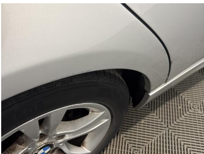
13: Qtr Panel osr Dented With Paint Damage
