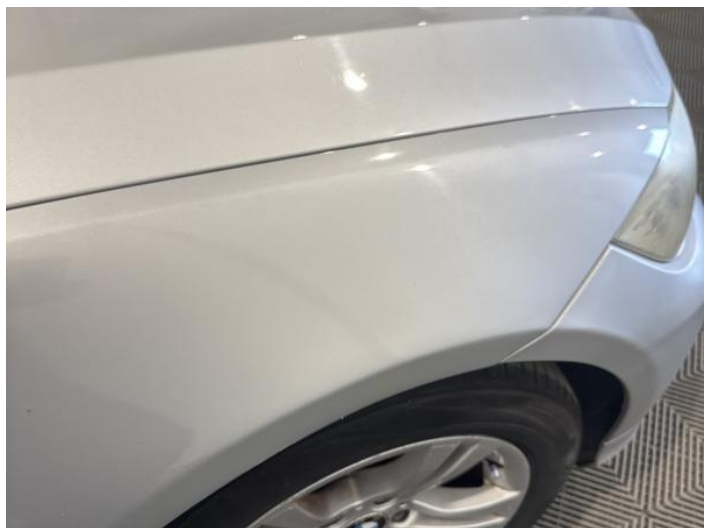
20: Wing osf Poor Previous Repair Poor Paint
