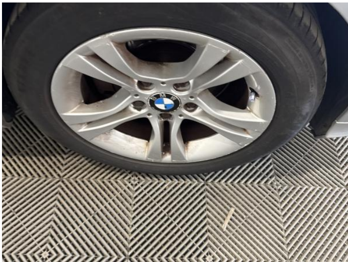
21: Wheel osf Scratched Over 50mm
