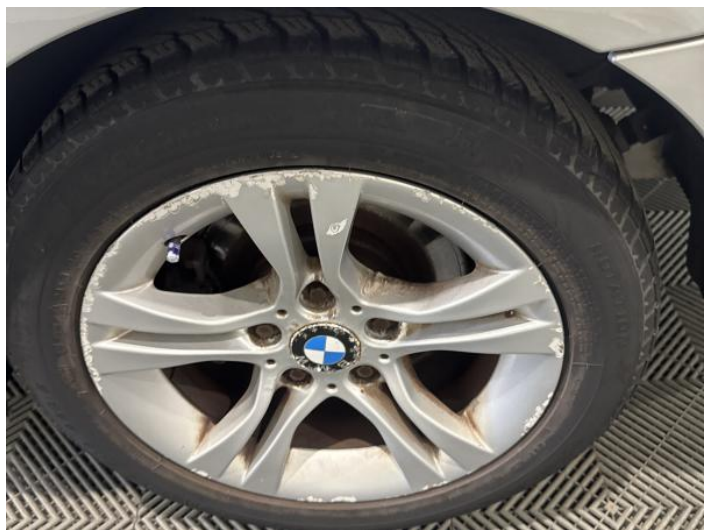
8: Wheel nsr Scratched Over 50mm
