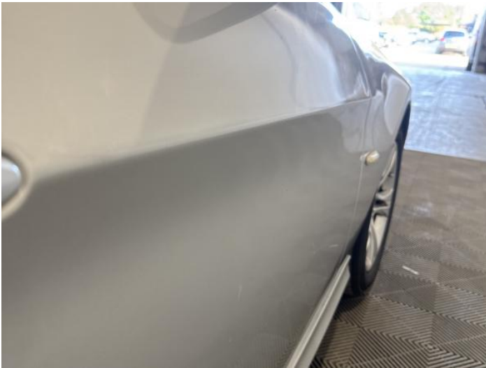
17: Door osf Dented With Paint Damage
