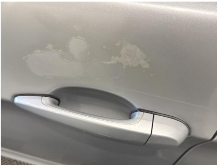
5: Door nsf Poor Previous Repair Poor Paint
