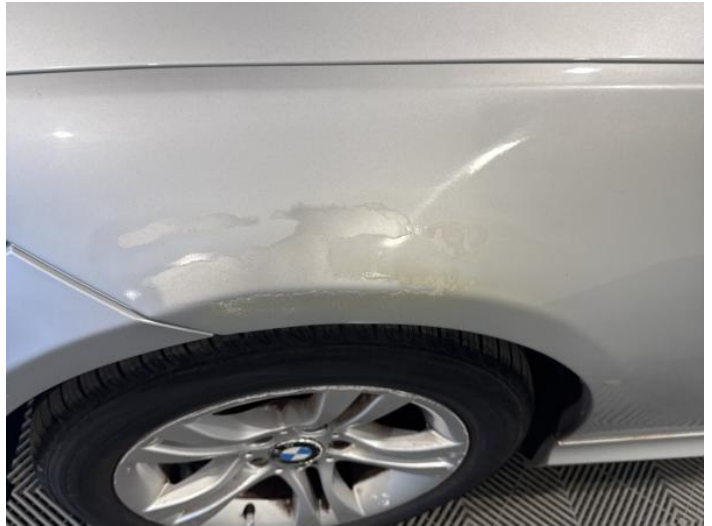
4: Wing nsf Poor Previous Repair Poor Paint
