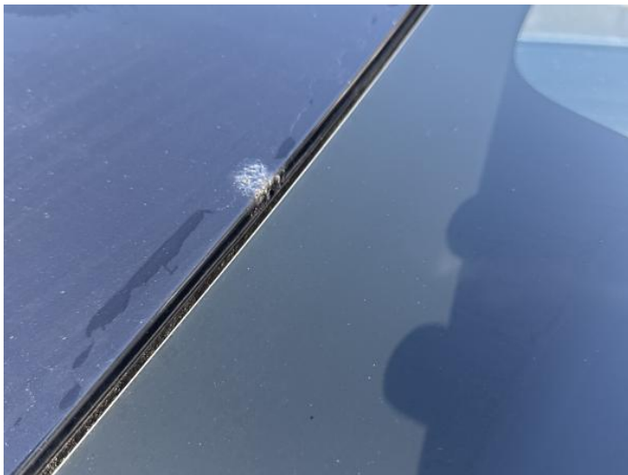
21: Roof Rusted Over 5mm
