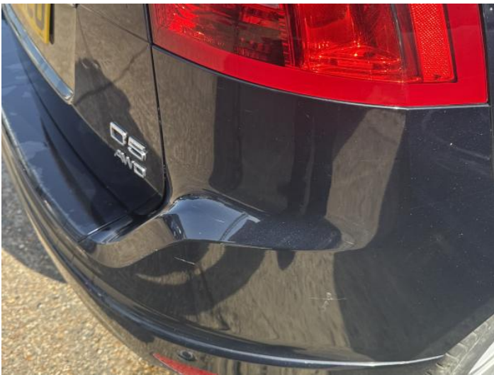
11: Bumper Rear Scratched Over 100mm Thru Paint
