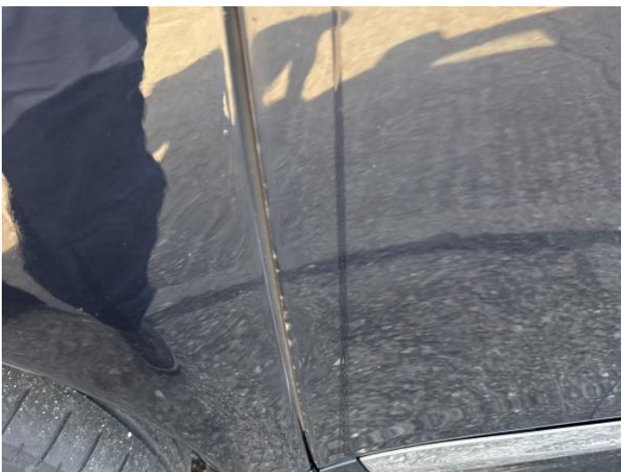
19: Door nsf Rusted Over 5mm
