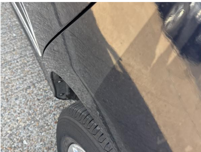
13: Qtr Panel nsr Dented Between 10mm + 30mm
