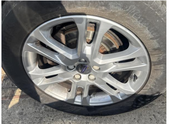
10: Wheel osr Scratched Over 50mm
