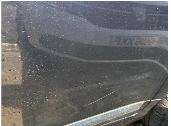
6: Door osf Scratched Over 25mm Thru Paint
