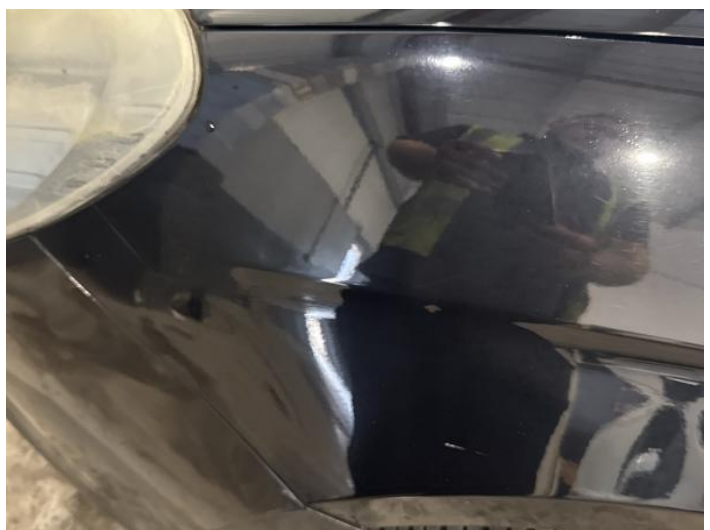
8: Wing nsf Dented With Paint Damage
