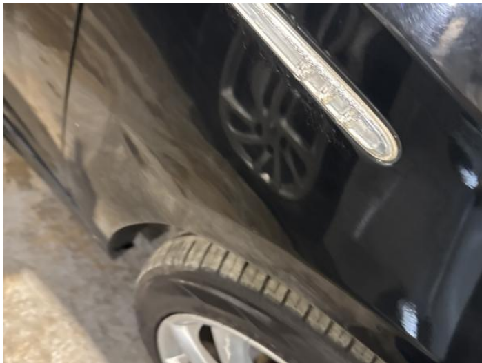
11: Wing osf Dented Over 30mm
