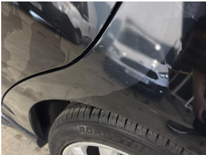
3: Qtr Panel nsr Poor Previous Repair Poor Paint
