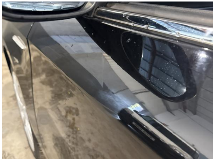
6: Door nsf Dented Between 10mm + 30mm
