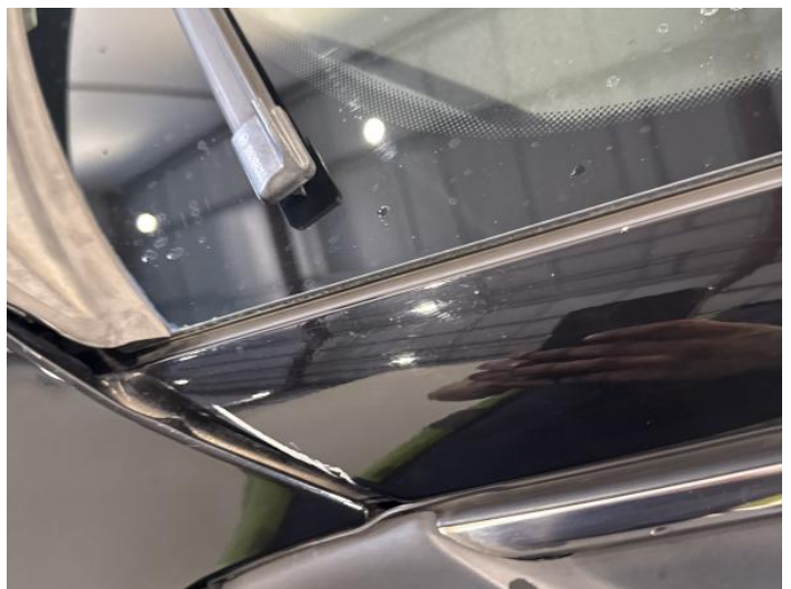
20: A Post ns Scratched Over 25mm Thru Paint
