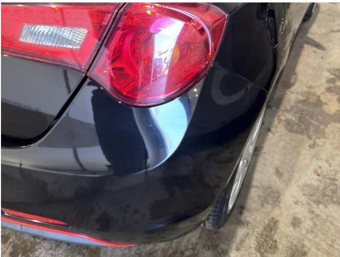
1: Bumper Rear Chipped Multiple Chips
