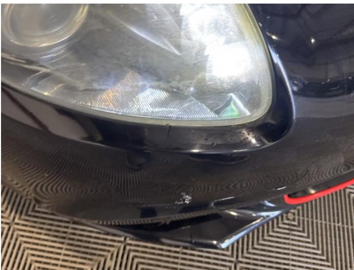
19: Bumper Front Cracked UpTo 25mm
