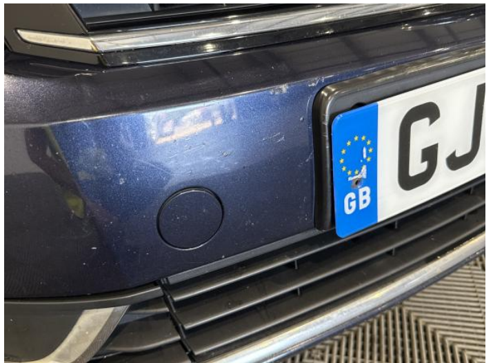
2: Bumper Front Scratched Over 100mm Thru Paint
