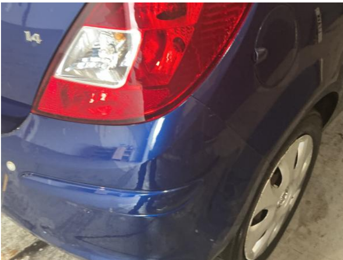
1: Bumper Rear Dented With Paint Damage
