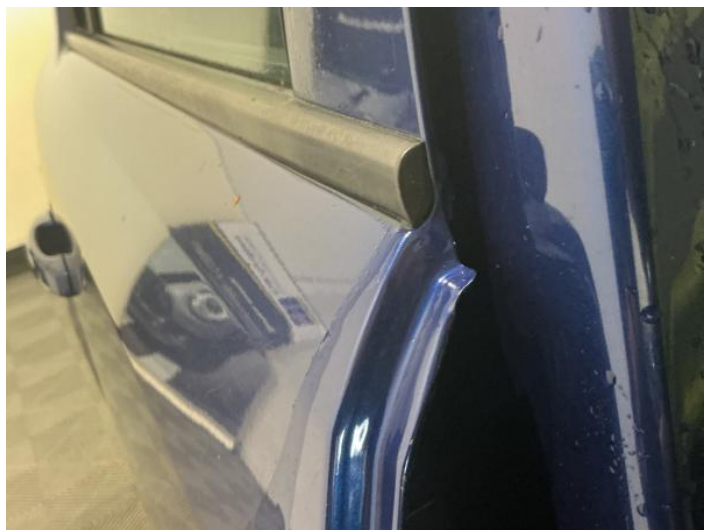
20: Door osr Poor Previous Repair Poor Paint
