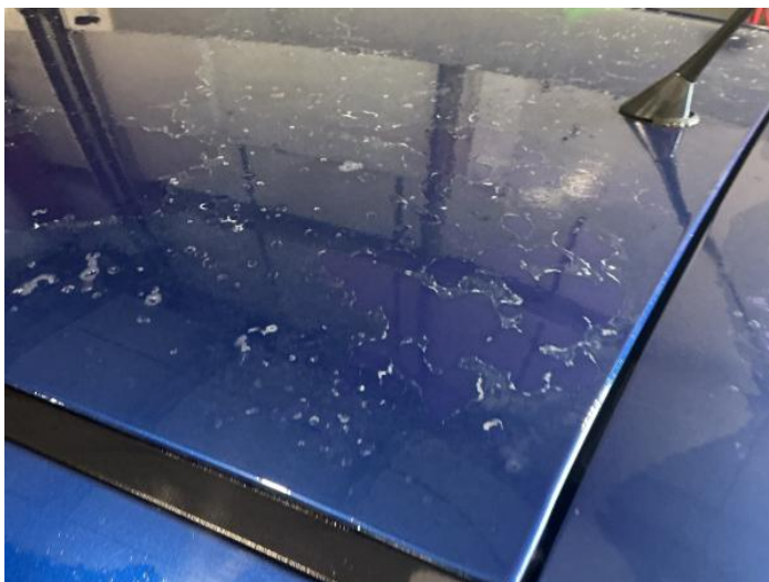
4: Roof Poor Previous Repair Paint Flake
