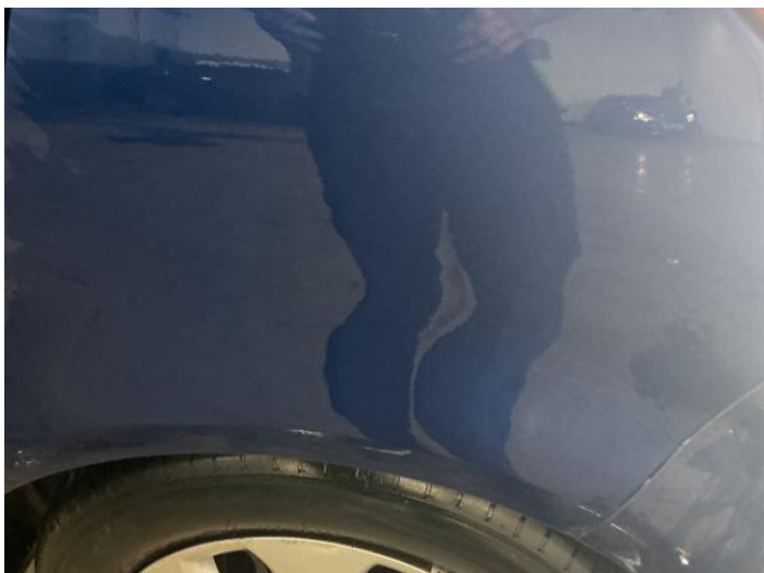
3: Qtr Panel nsr Dented With Paint Damage
