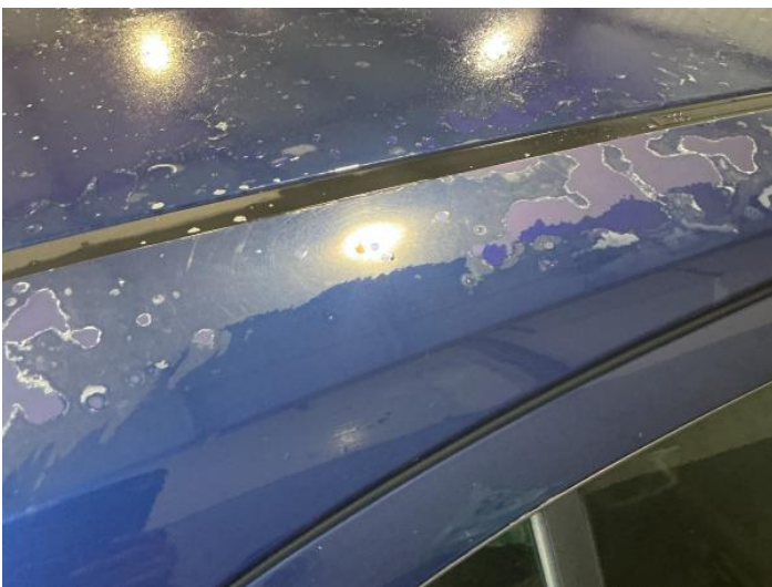
19: D Post os Poor Previous Repair Paint Flake
