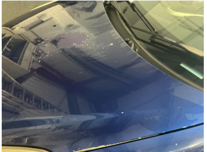
10: Bonnet Dented With Paint Damage
