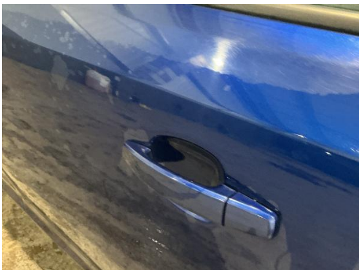
5: Door nsr Dented 2 Or Less UpTo 10mm
