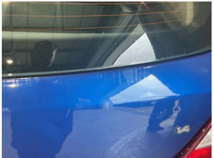
2: Boot Lid Dented With Paint Damage
