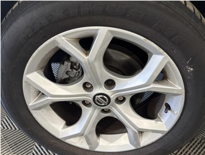
3: Wheel nsf Scratched Over 50mm
