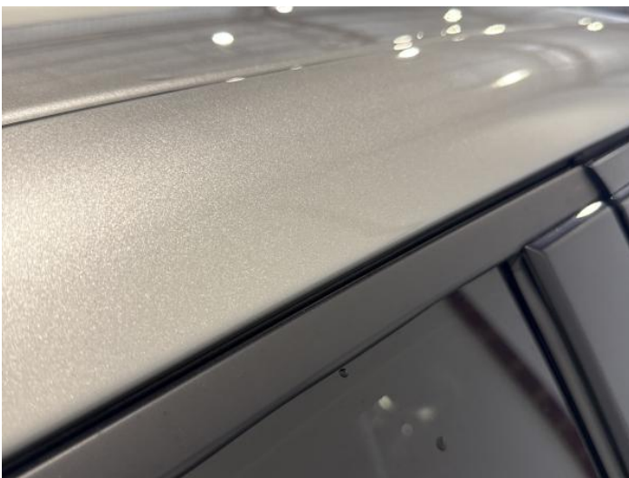
7: B Post os Dented Between 10mm + 30mm
