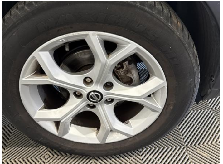
10: Wheel osf Scratched Over 50mm
