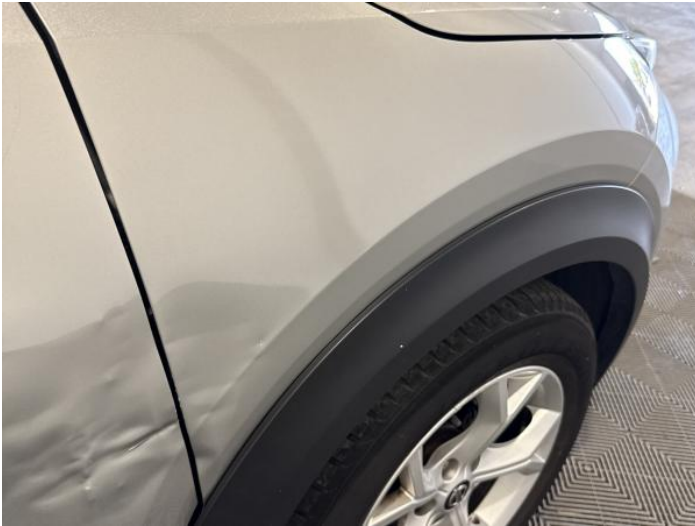
9: Wing osf Dented Over 30mm
