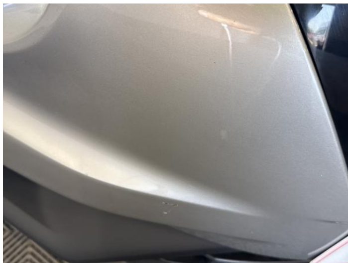
2: Bumper Front Scratched 25 to 100mm Thru Paint
