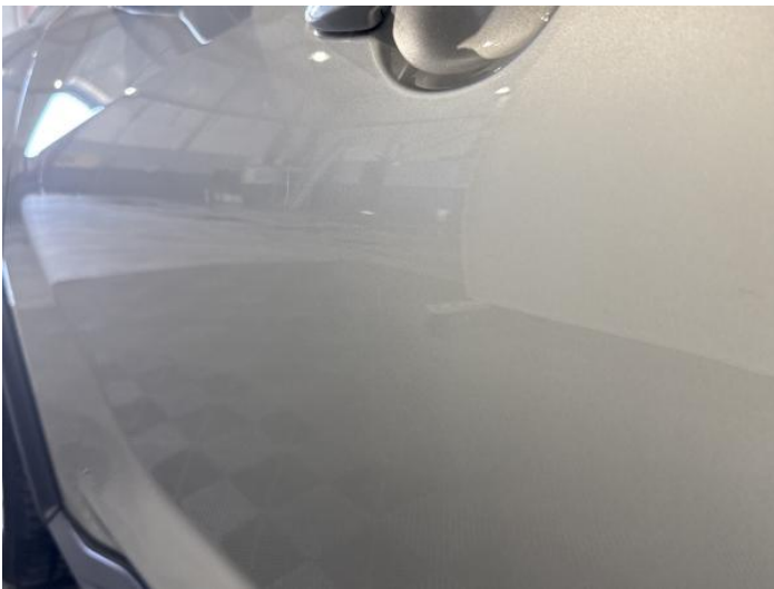
5: Door nsf Poor Previous Repair Rippled UpTo 30%
