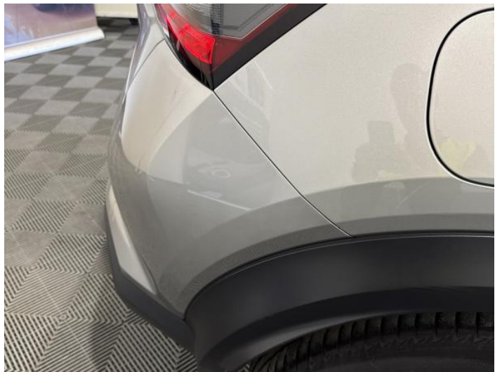
6: Bumper Rear Poor Previous Repair Poor Colour
