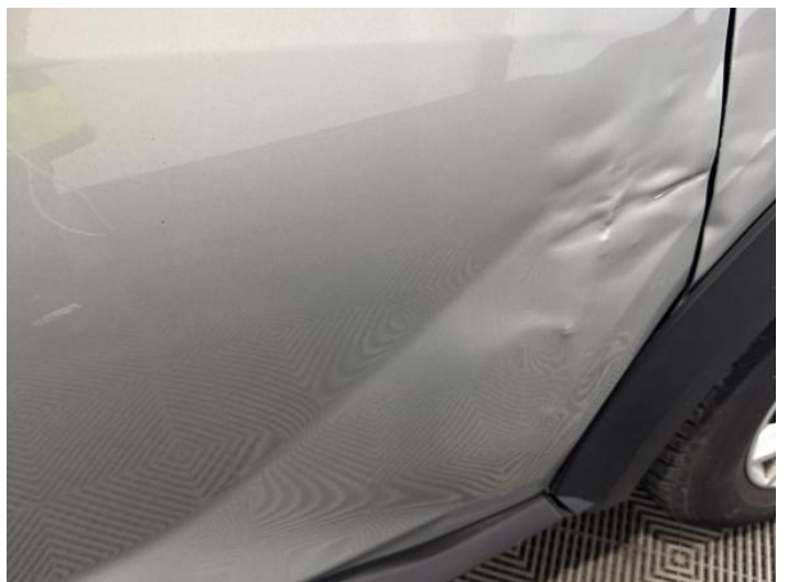
8: Door osf Dented Over 30mm
