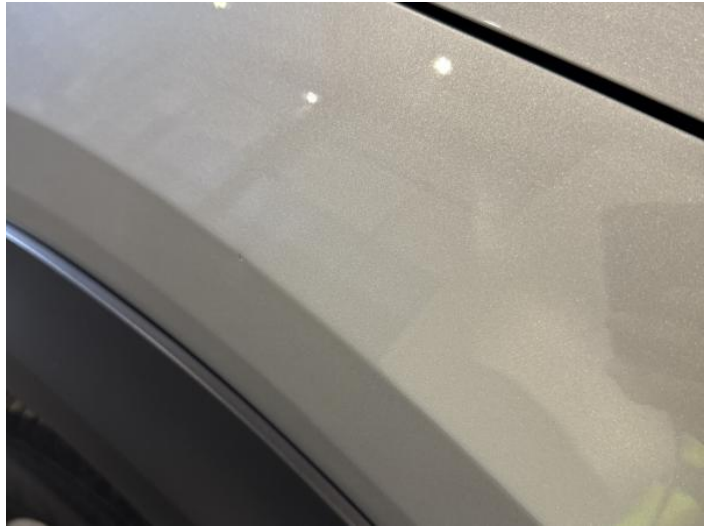
4: Wing nsf Dented Between 10mm + 30mm
