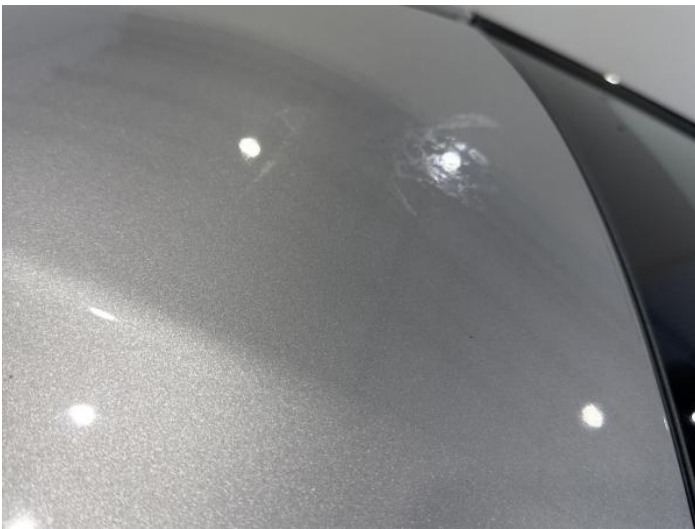
11: Roof Scratched Over 25mm Thru Paint
