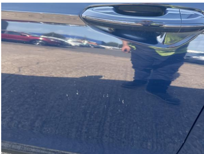
7: Door nsf Chipped Multiple Chips
