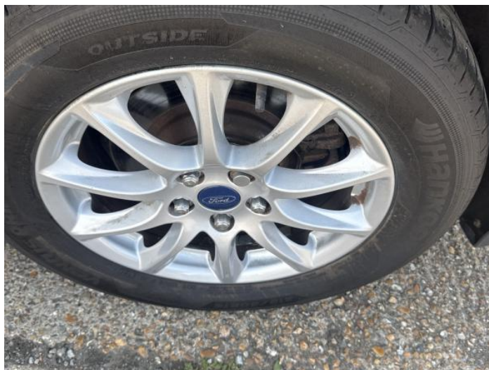
10: Wheel nsr Scratched Over 50mm
