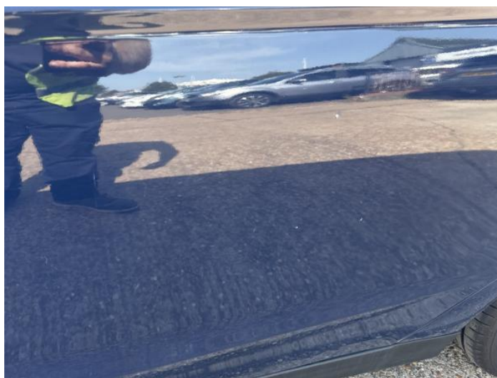
8: Door nsr Poor Previous Repair Poor Paint
