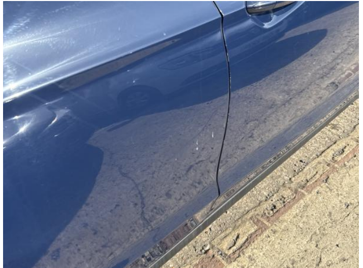
16: Door osf Dented With Paint Damage
