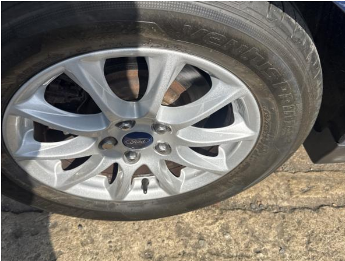
15: Wheel osf Scratched Over 50mm
