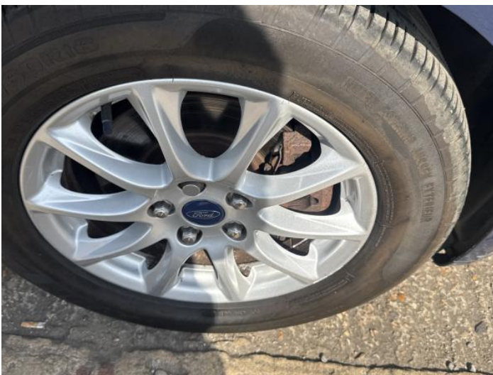
19: Wheel osf Scratched Up To 50mm
