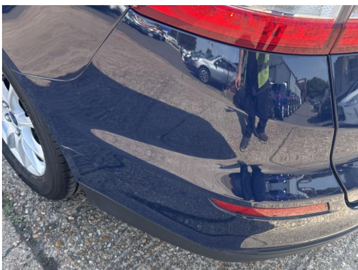
11: Bumper Rear Scratched 25 to 100mm Thru Paint
