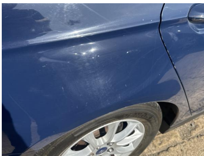
14: Qtr Panel osr Dented With Paint Damage
