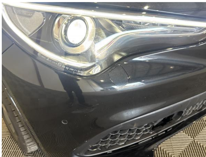
2: Bumper Front Scratched Over 100mm Thru Paint
