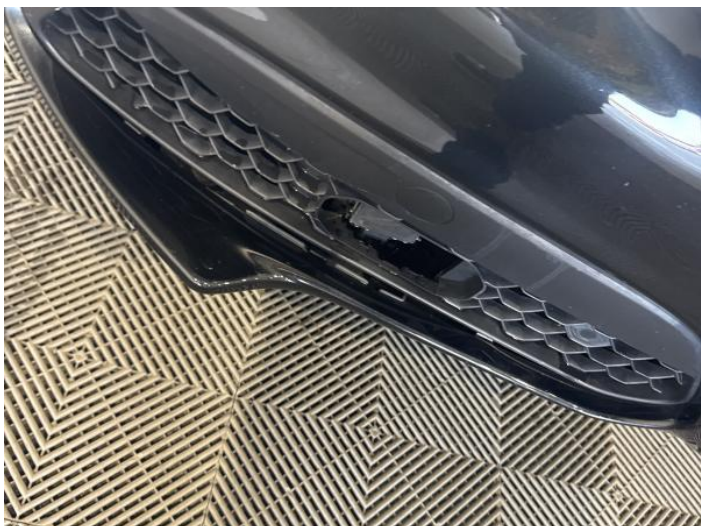
3: Bumper Front Moulding Broken Replace
