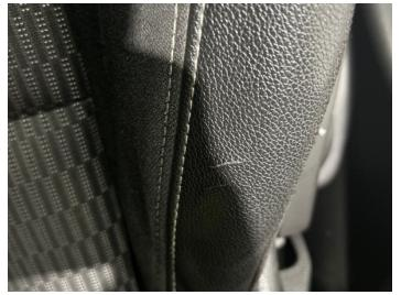
11: Seat Base Cover osf Torn UpTo 3mm
