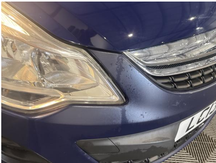
3: Bumper Front Poor Previous Repair Poor Paint
