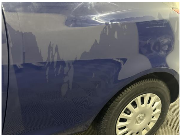
8: Qtr Panel nsr Dented With Paint Damage
