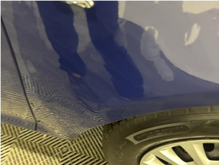
15: Wing osf Dented Over 2 UpTo 10mm
