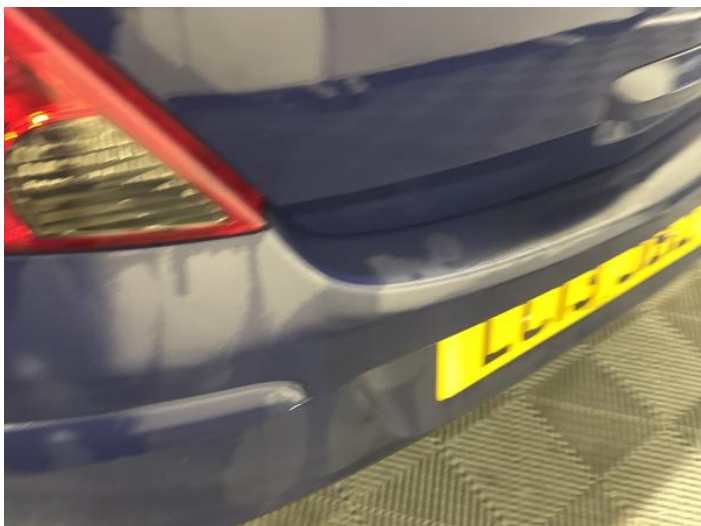
9: Bumper Rear Poor Previous Repair Poor Paint
