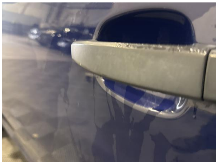
6: Door nsf Dented Over 2 UpTo 10mm
