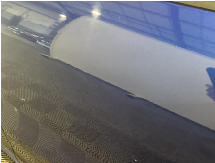
9: Door nsr Dented Between 10mm + 30mm
