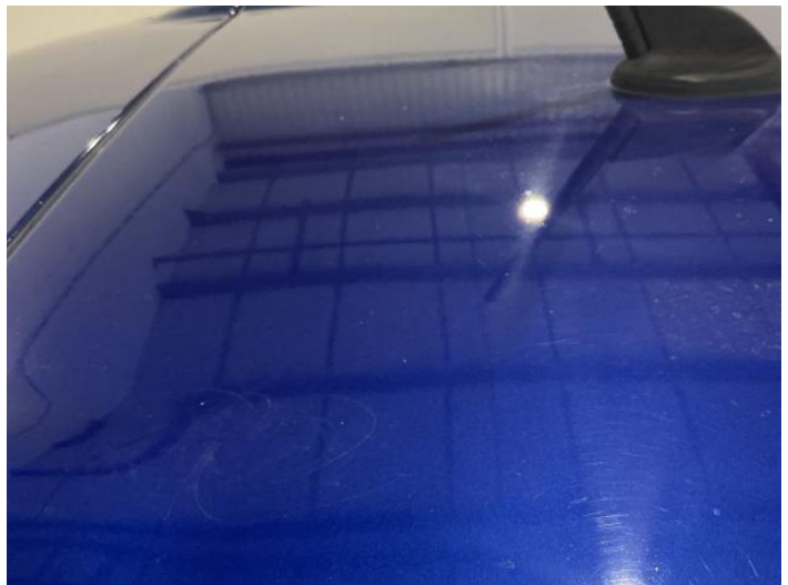
22: Roof Dented Between 10mm + 30mm
