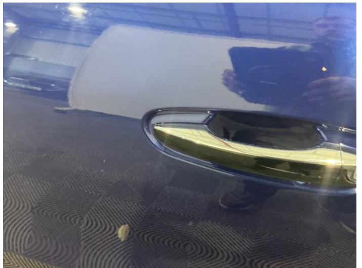
6: Door nsf Dented Between 10mm + 30mm
