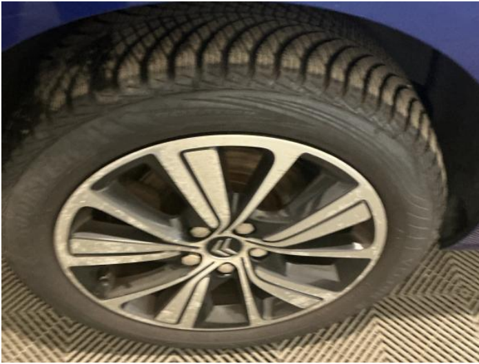
15: Wheel osr Scratched Over 50mm
