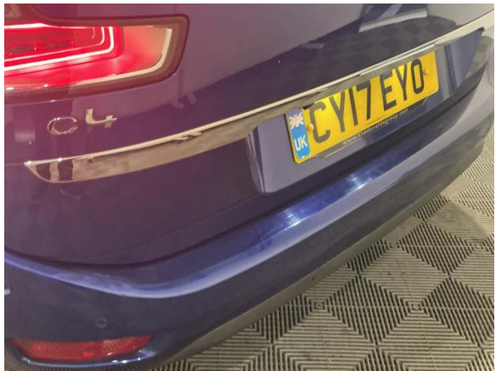
12: Bumper Rear Poor Previous Repair Rippled UpTo 30%
