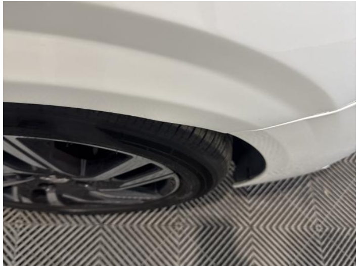
22: Wing osf Dented Between 10mm + 30mm
