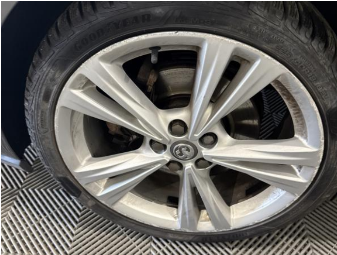
3: Wheel osf Scratched Over 50mm
