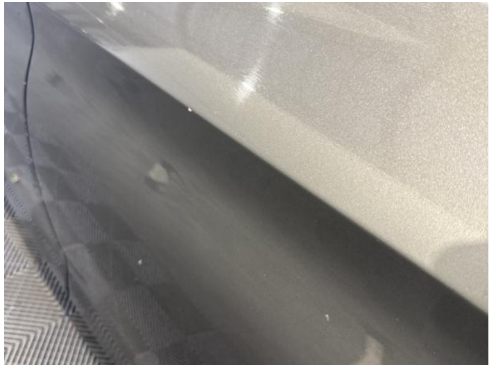
6: Door osr Scratched Over 25mm Thru Paint
