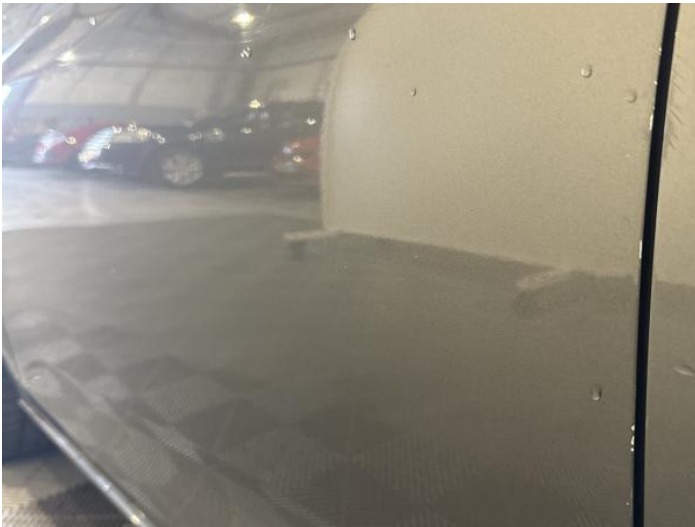
5: Door osf Dented Between 10mm + 30mm
