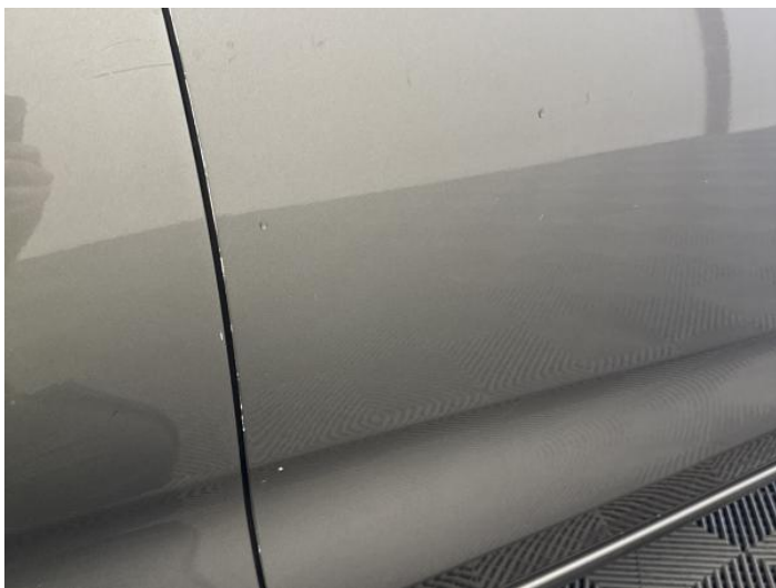
13: Door osf Scratched Over 25mm Thru Paint
