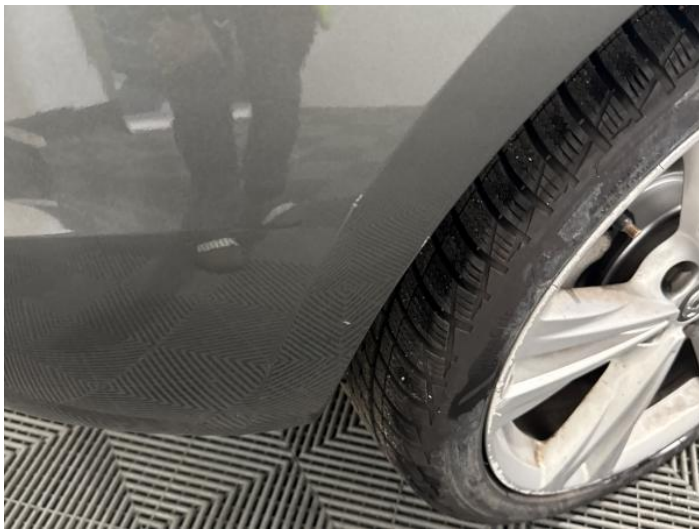
9: Bumper Rear Scratched 25 to 100mm Thru Paint
