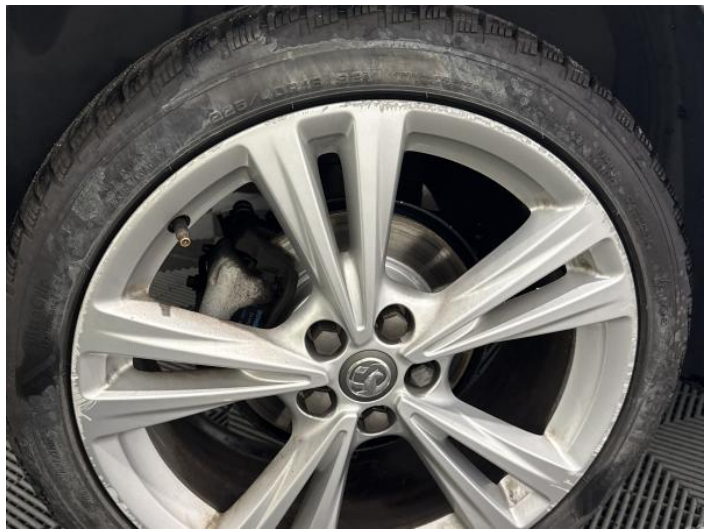
10: Wheel osr Scratched Over 50mm
