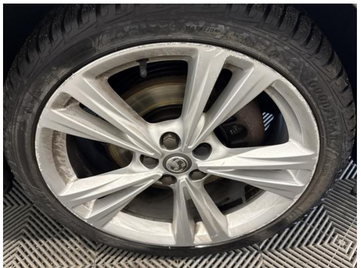
14: Wheel osf Scratched Over 50mm
