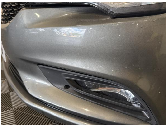
2: Bumper Front Chipped Multiple Chips
