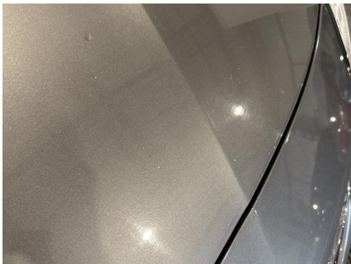
1: Bonnet Dented With Paint Damage
