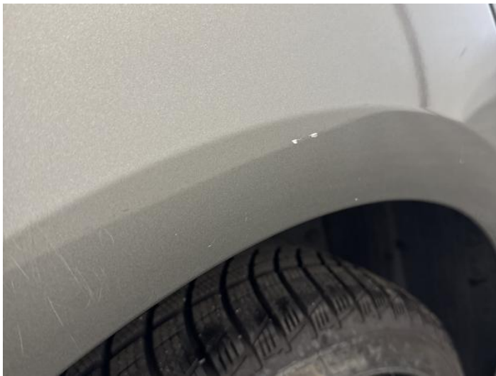
11: Qtr Panel osr Dented With Paint Damage
