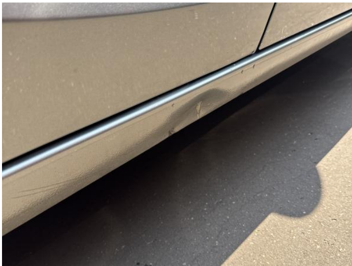
17: Sill os Dented Over 30mm
