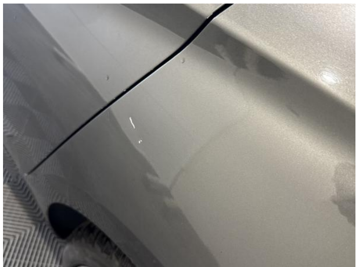
8: Qtr Panel nsr Dented With Paint Damage
