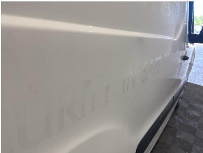
9: Qtr Panel osr Dented Over 30mm
