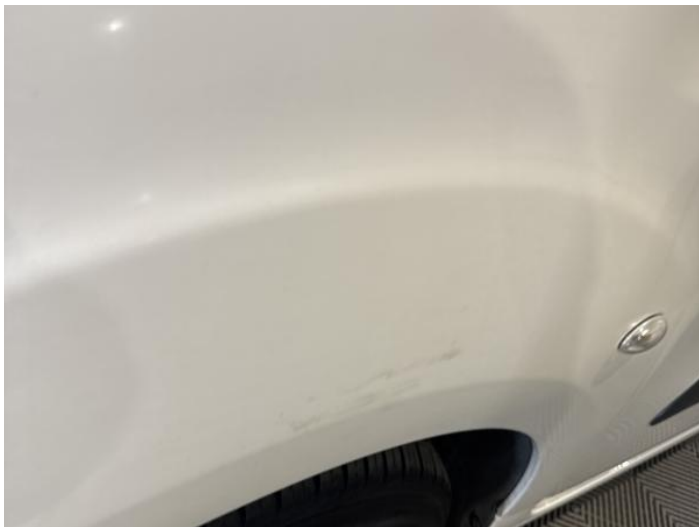
3: Wing nsf Poor Previous Repair Poor Paint
