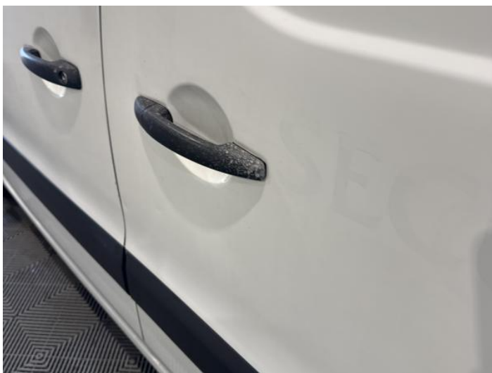
5: Door nsr Dented Over 30mm
