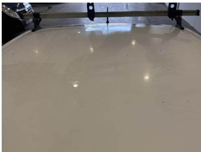
8: Roof Dented Over 30mm
