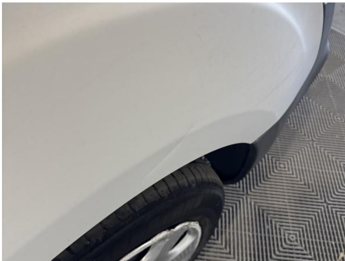
11: Wing osf Dented Over 30mm
