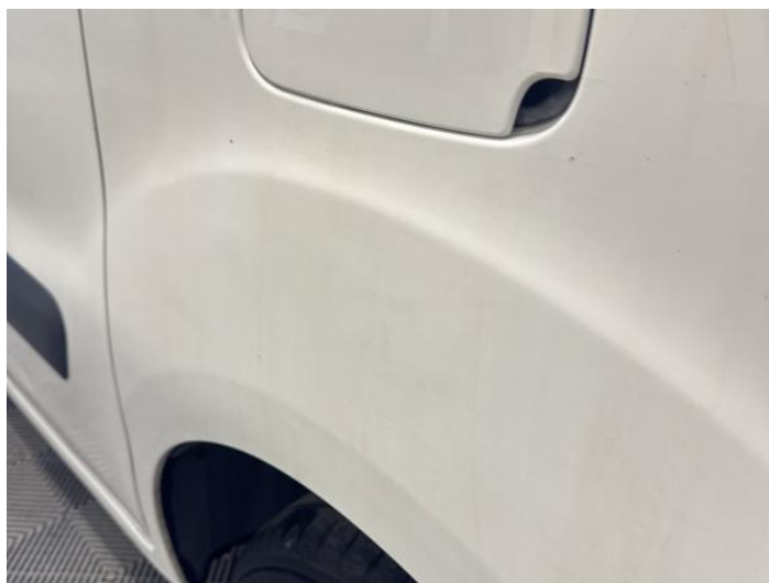
6: Qtr Panel nsr Dented Over 30mm
