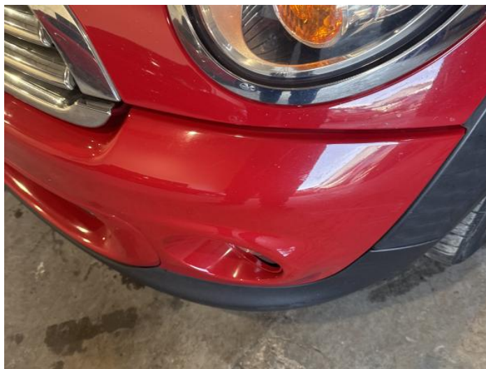
2: Bumper Front Scratched 25 to 100mm Thru Paint
