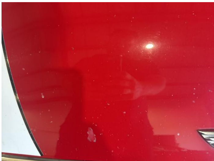
1: Bonnet Poor Previous Repair Paint Flake
