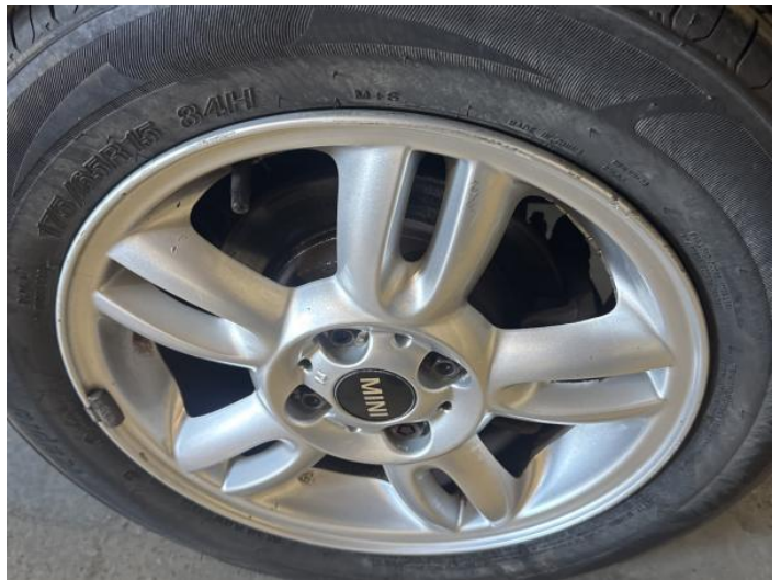
12: Wheel nsr Scratched Over 50mm
