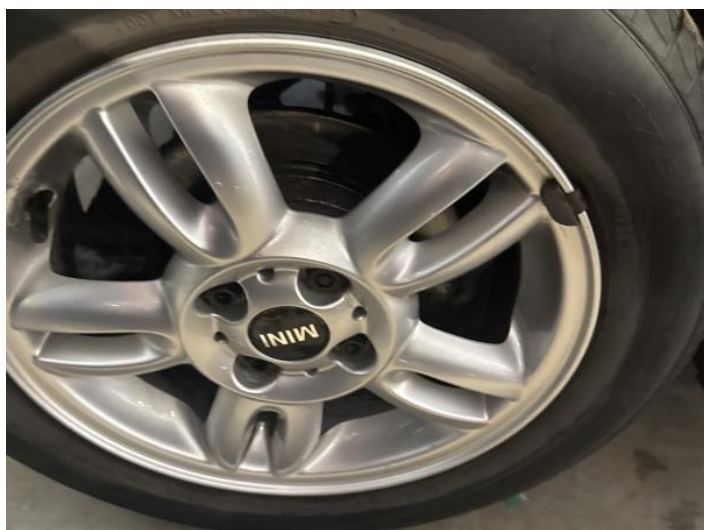
8: Wheel osr Scratched Over 50mm
