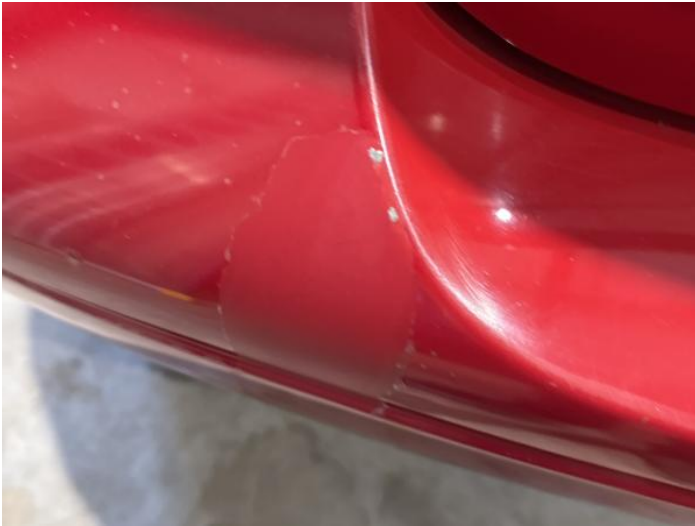
9: Bumper Rear Poor Previous Repair Paint Flake
