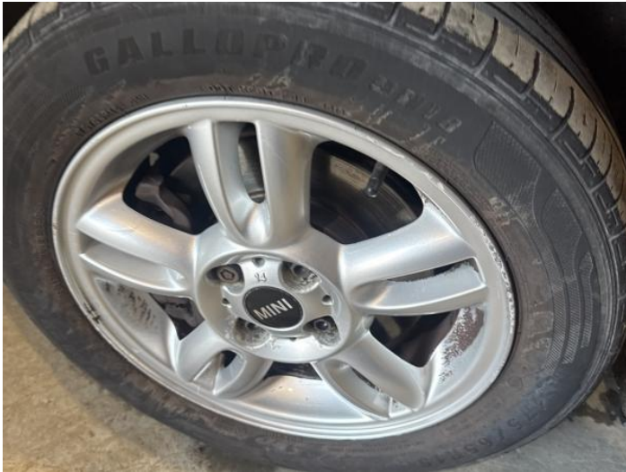
16: Wheel nsf Scratched Over 50mm
