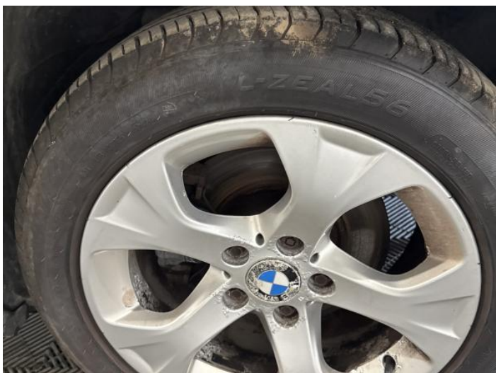
23: Wheel osf Scratched Up To 50mm
