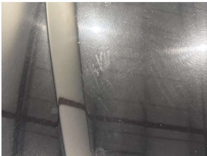
1: Bonnet Poor Previous Repair Poor Paint
