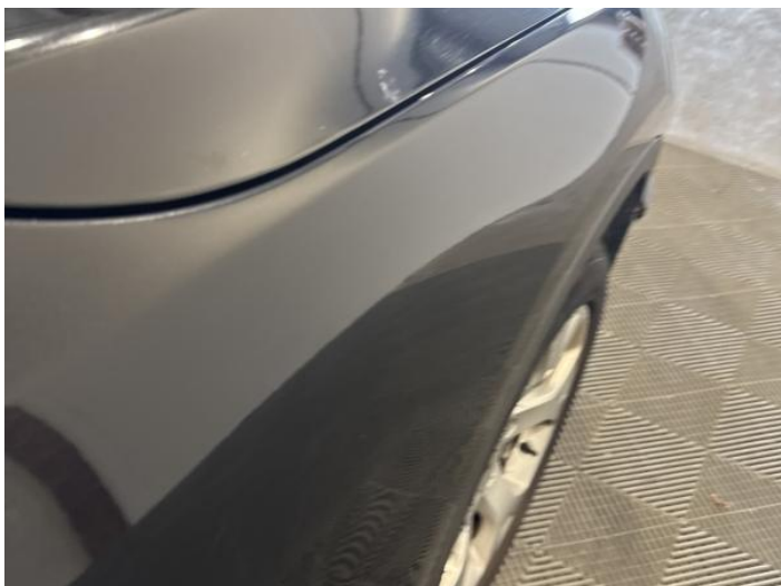
21: Wing osf Dented With Paint Damage
