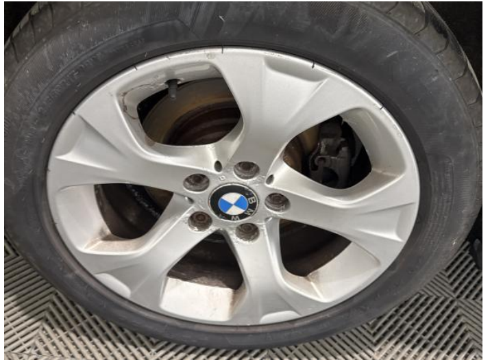
16: Wheel osr Scratched Over 50mm
