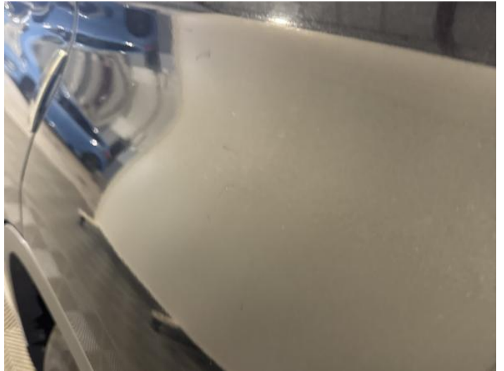
10: Qtr Panel nsr Dented Over 2 UpTo 10mm
