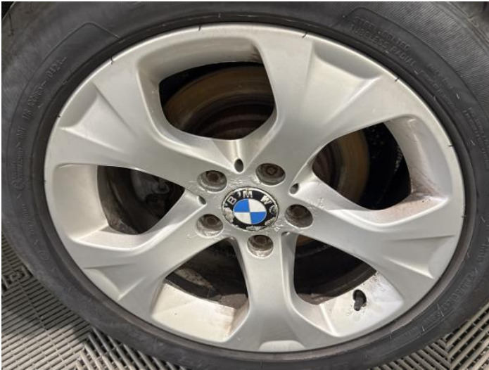
9: Wheel nsr Scratched Over 50mm
