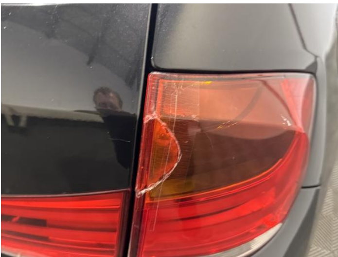
13: Lamp osr Broken Replace
