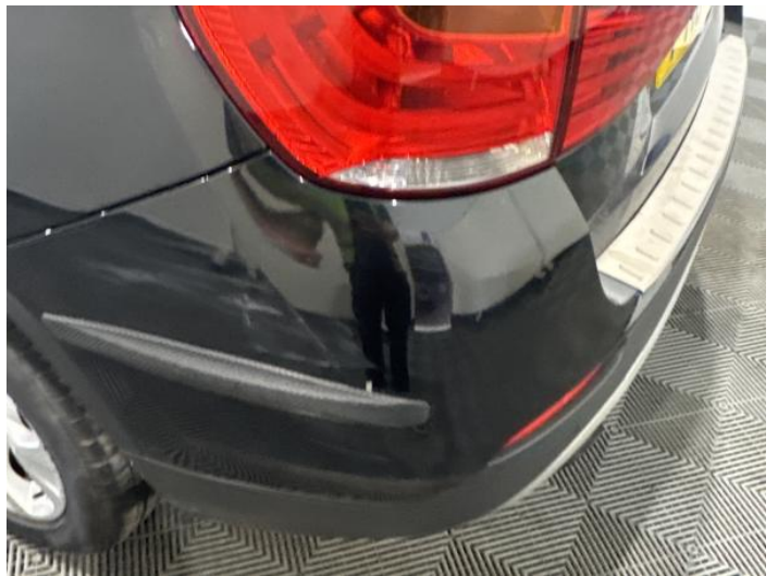
12: Bumper Rear Scratched Over 100mm Thru Paint
