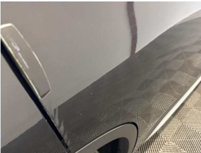
17: Door osr Poor Previous Repair Poor Paint
