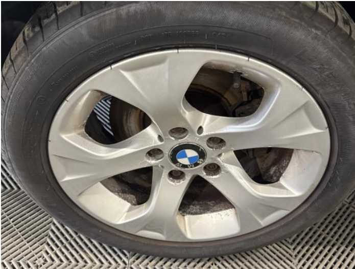
3: Wheel nsf Corroded Light
