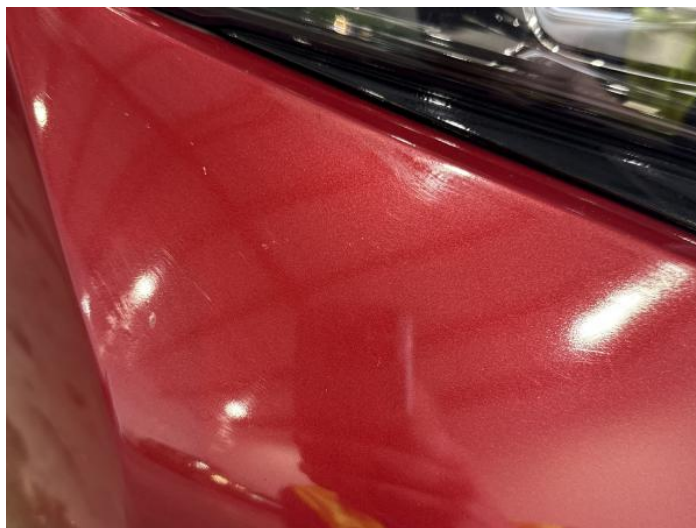
2: Bumper Front Poor Previous Repair Poor Paint
