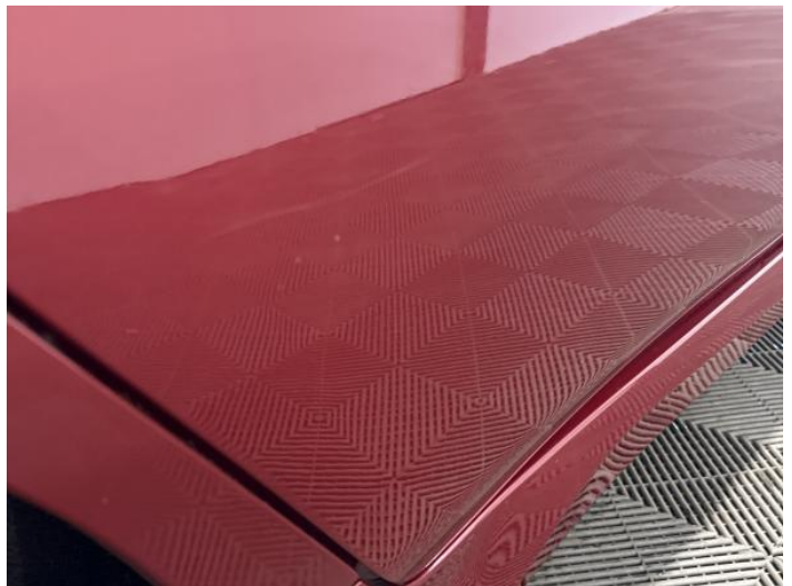
10: Door osr Scratched Over 25mm Thru Paint
