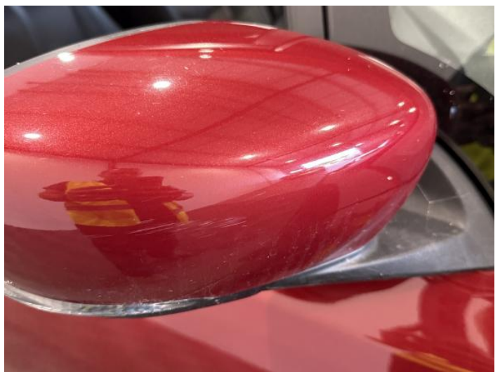
12: Door Mirror Assy osf Scratched (Painted) Over 25mm Thru Paint
