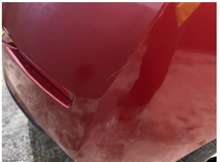
8: Bumper Rear Scratched 25 to 100mm Thru Paint
