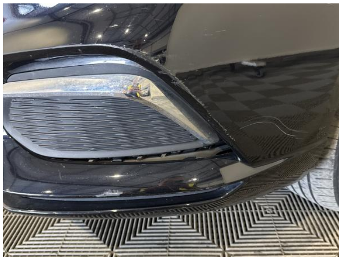
2: Bumper Front Scratched Over 100mm Thru Paint
