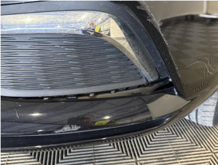
3: Bumper Front Moulding Scuffed (Unpainted) Over 100mm
