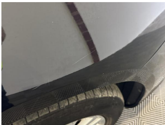
14: Wing osf Scratched Over 25mm Thru Paint
