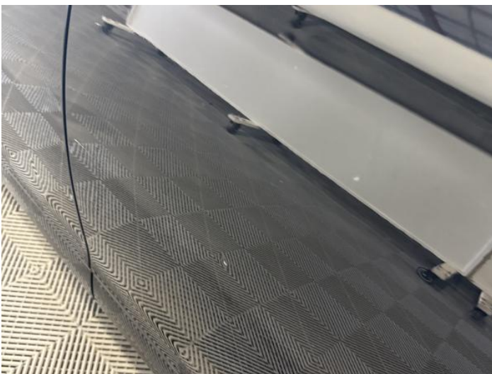
7: Door nsr Dented With Paint Damage
