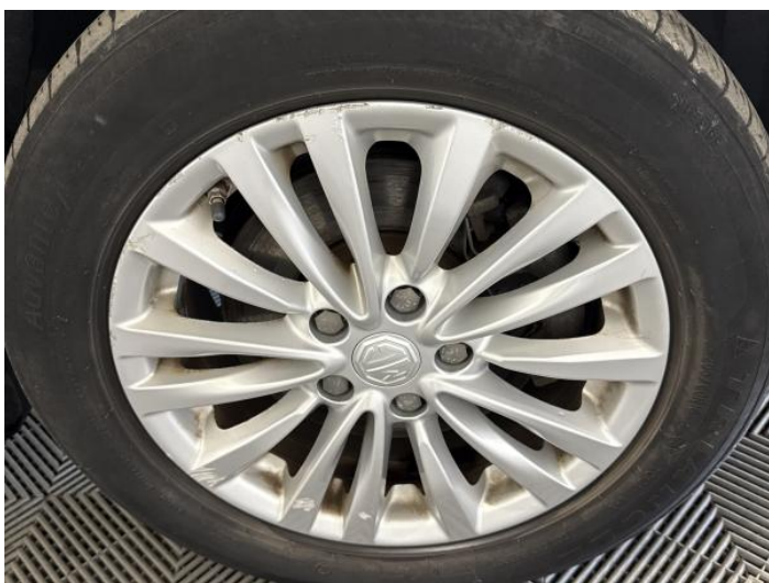
13: Wheel osf Scratched Over 50mm
