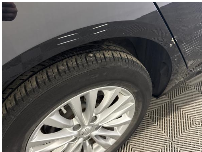
10: Qtr Panel osr Dented With Paint Damage
