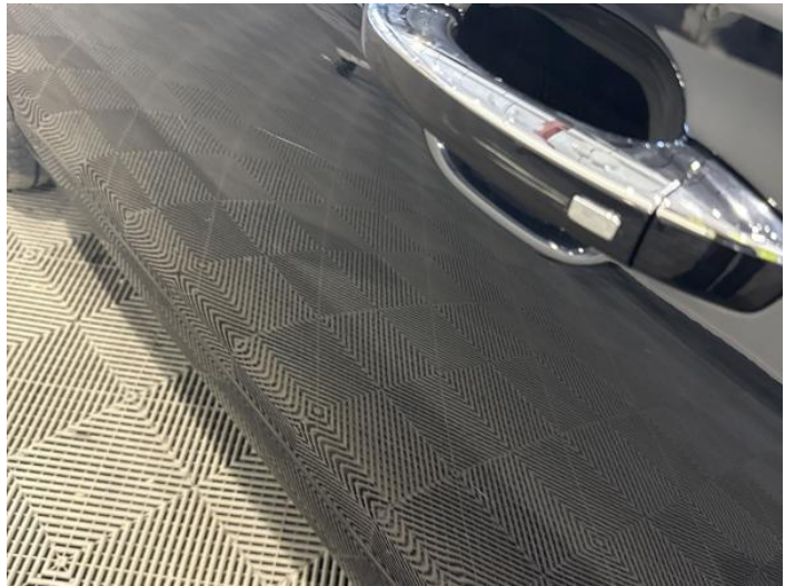
6: Door nsf Scratched Over 25mm Thru Paint
