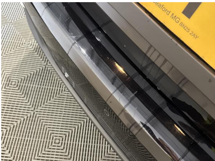
9: Bumper Rear Scratched 25 to 100mm Thru Paint
