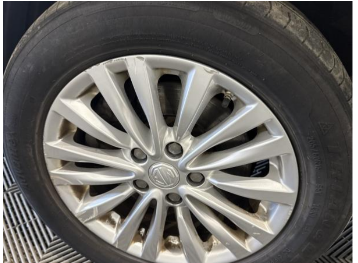
4: Wheel nsf Scratched Over 50mm
