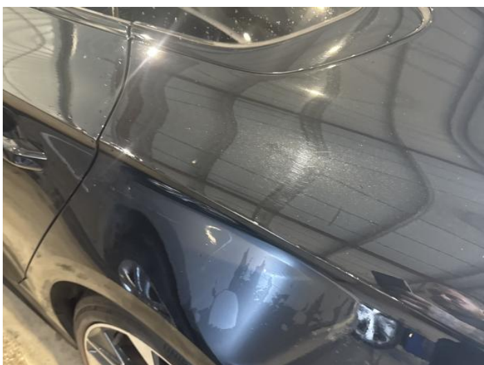
5: Qtr Panel nsr Dented With Paint Damage
