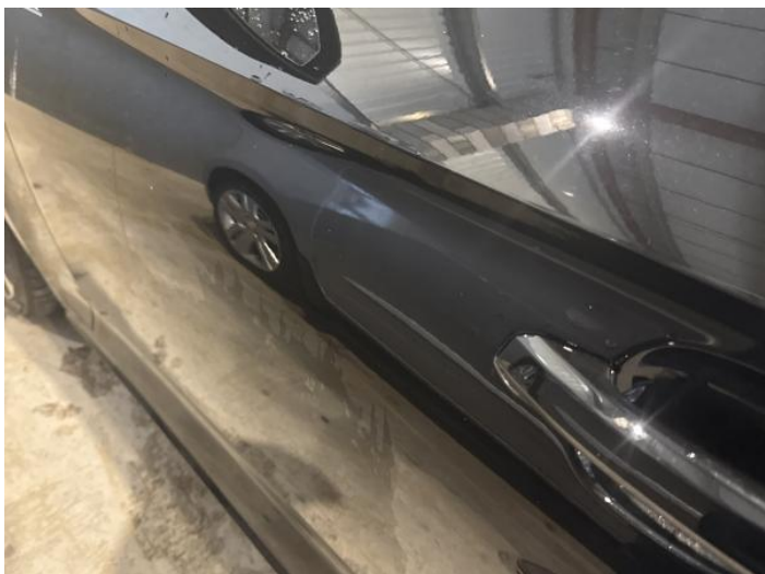
9: Door nsf Dented Over 2 UpTo 10mm
