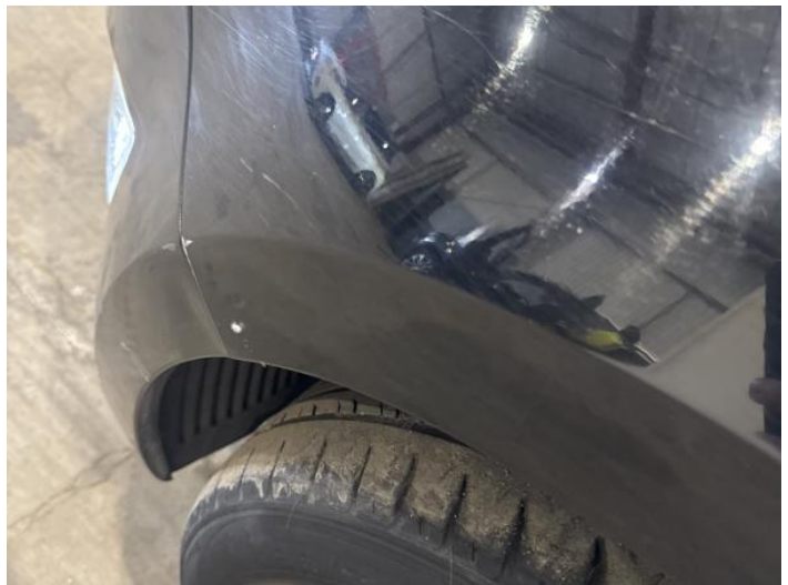
18: Wing nsf Scratched Over 25mm Thru Paint
