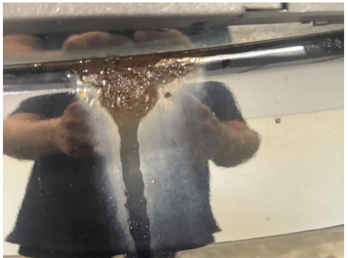
12: Boot Lid Rusted Over 5mm
