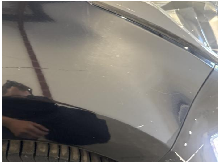
4: Wing osf Scratched Over 25mm Thru Paint
