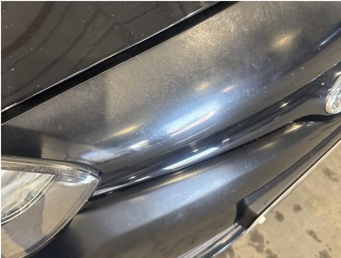
3: Bumper Front Poor Previous Repair Poor Paint
