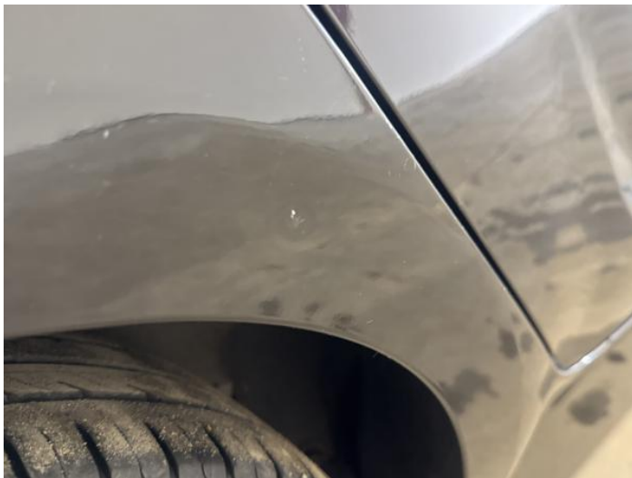
9: Qtr Panel osr Dented With Paint Damage
