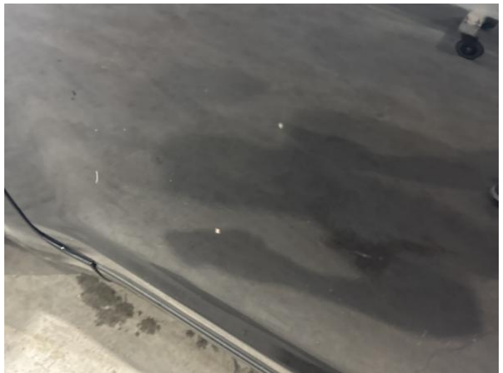
16: Door nsf Chipped Multiple Chips
