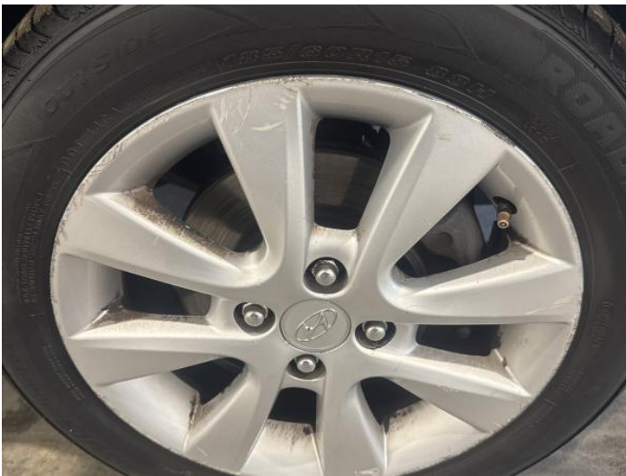
5: Wheel osf Scratched Over 50mm
