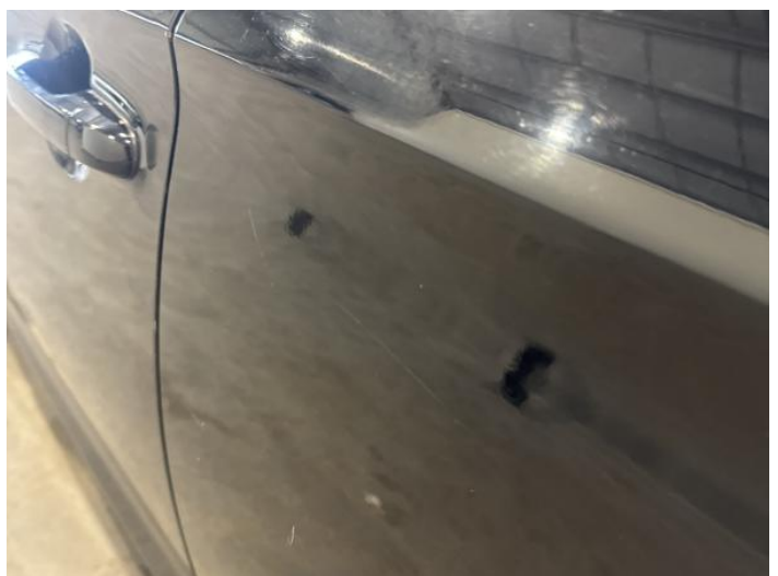
14: Door nsr Dented With Paint Damage
