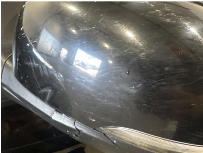
17: Door Mirror Assy nsf Broken Replace
