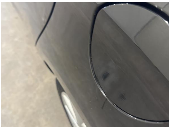
13: Qtr Panel nsr Dented With Paint Damage
