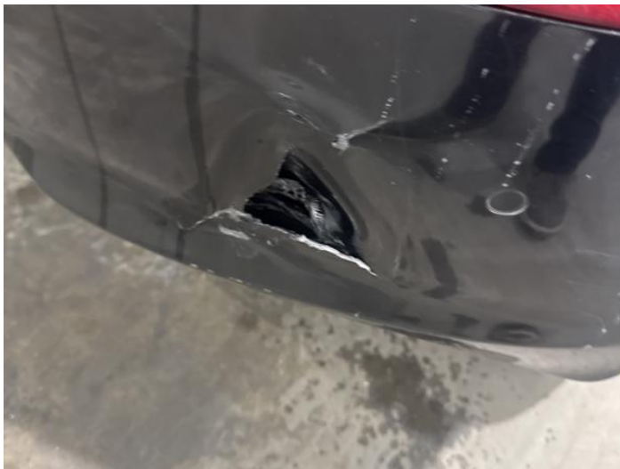
11: Bumper Rear Hole Over 25mm
