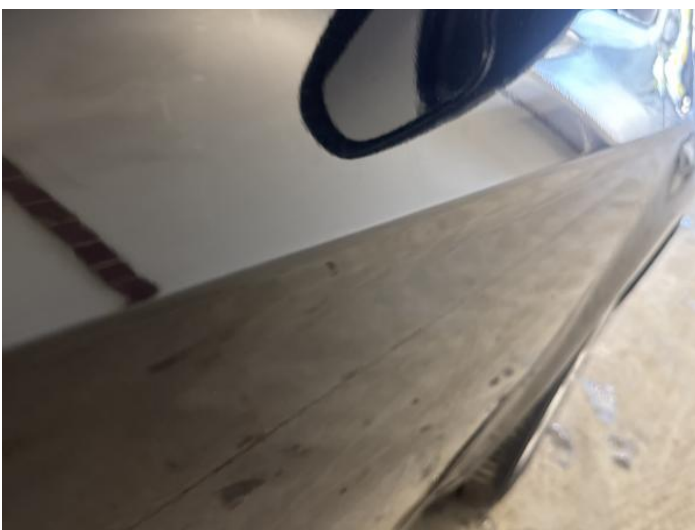
7: Door osf Dented Between 10mm + 30mm
