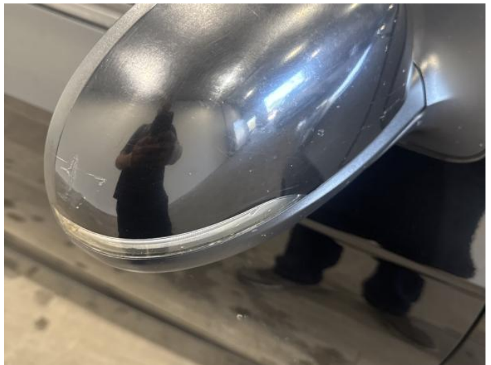
6: Door Mirror Assy osf Scratched (Painted) Over 25mm Thru Paint
